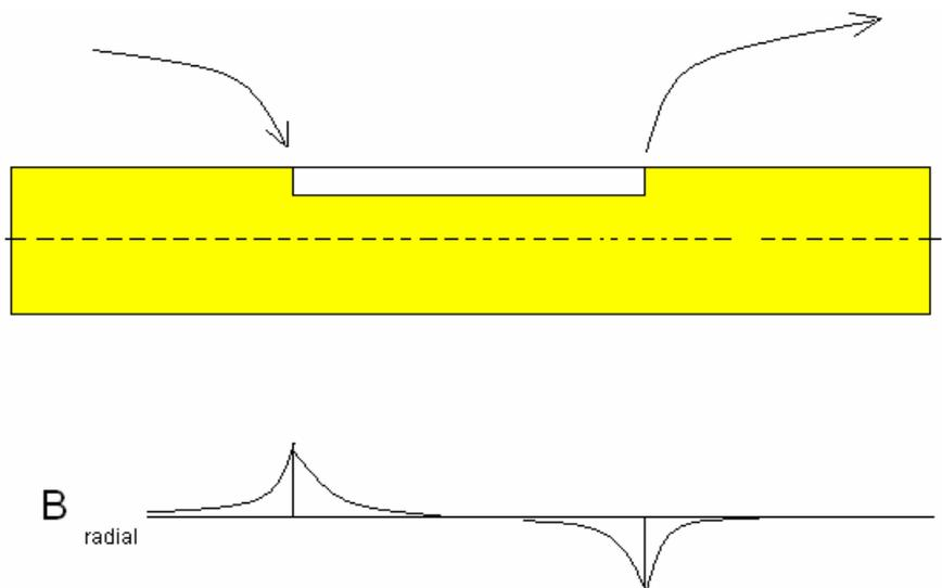
Fig. 3: Radial flux entering the bar at the beginning and leaving it at the end of the crack.
