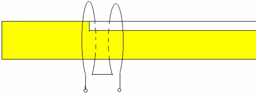
Fig. 2: Two differentially connected loops of pair of secondary coils.
