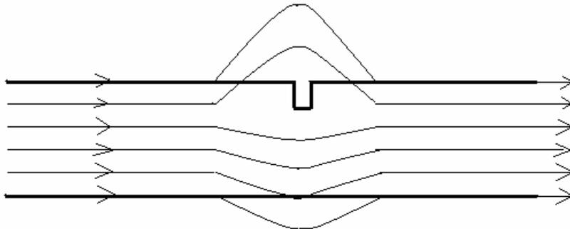
Fig. 4: Magnetic leakage field in two dimensions.
