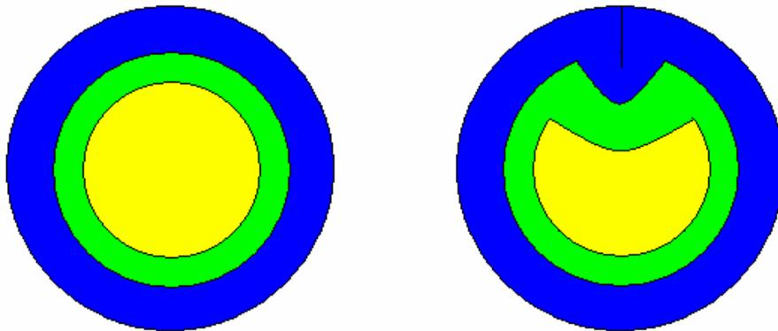
Fig. 1: Cross-section of a metal bar with a radial crack and without a crack.
