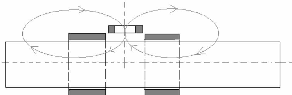
Fig. 5: Two parts of a magnetizing coil with one secondary coil in the middle.
