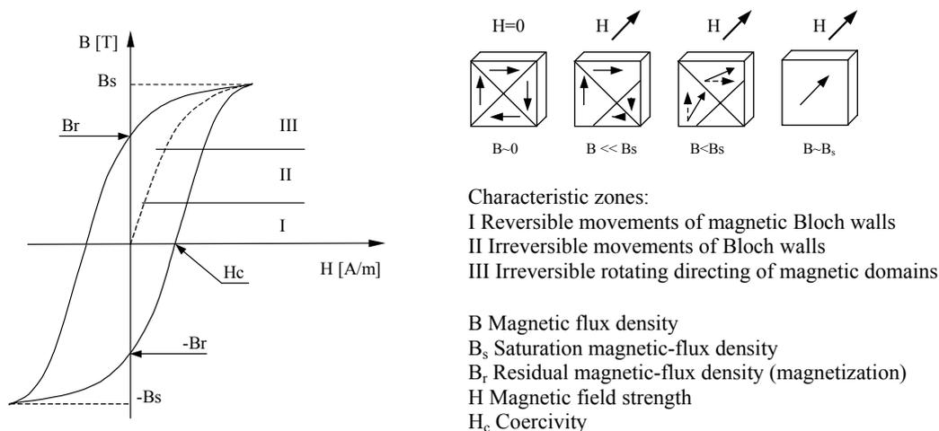
Fig. 1: Magnetization curve of ferromagnetic material with characteristic zones and values [6].
