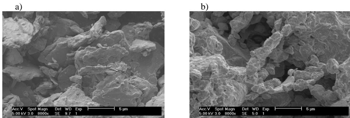
Fig. 5: SEM micrographs of Fe-Co powders prepared with mechanical alloying after milling time a) 12 hours: b) 36 hours.
