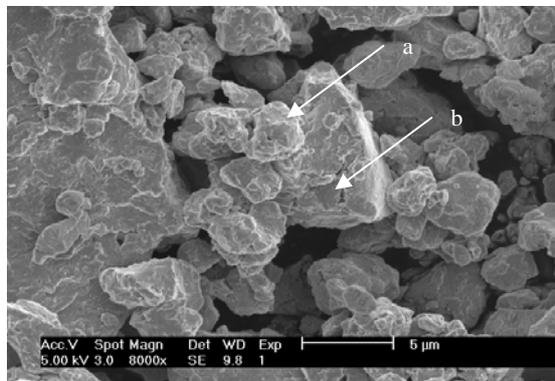
Fig. 4: Micrograph of Fe-Co powders shows welding (a) and fracture (b).
