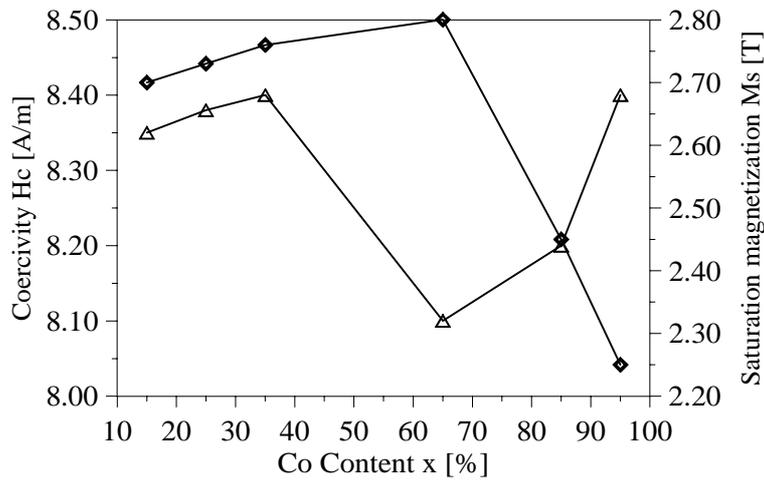
Fig. 1: Dependence of Co concentration on saturation magnetization Ms and coercivity Hc for MA Fe - Co powders after 36 hours milling time.
