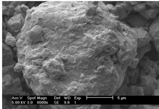
Fig. 3: Micrograph of unmixed Fe-Co powders.
