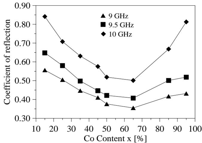
Fig. 2: Dependence of Co concentration upon the coefficient of reflection for MA Fe - Co powders after 36 hours milling time.
