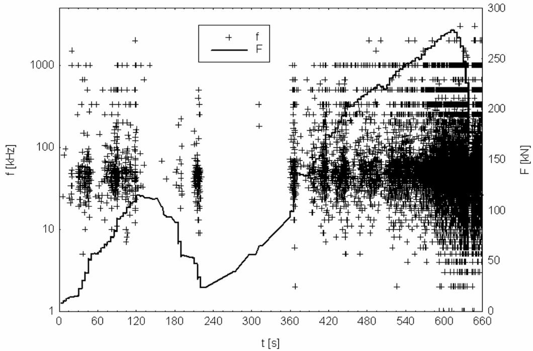
Fig. 4: Acoustic emission hits dependent on average frequency and time (dagger) and dependence force (solid curve) on time.
