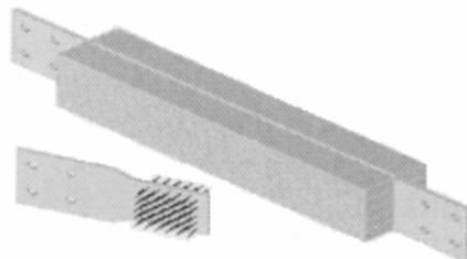
Fig. 1: Schematic representation of metal timber join.
