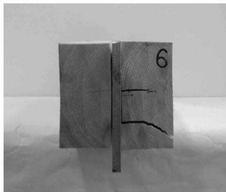
Fig. 11: The test specimen with crack after loading.
