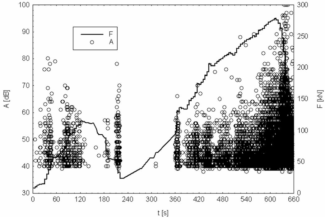
Fig. 5: Acoustic emission hits dependent on amplitude and time (circle) and dependence force (solid curve) on time.
