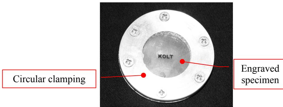
Fig. 3: Photograph of the clamped specimen with a laser-engraved inscription.
