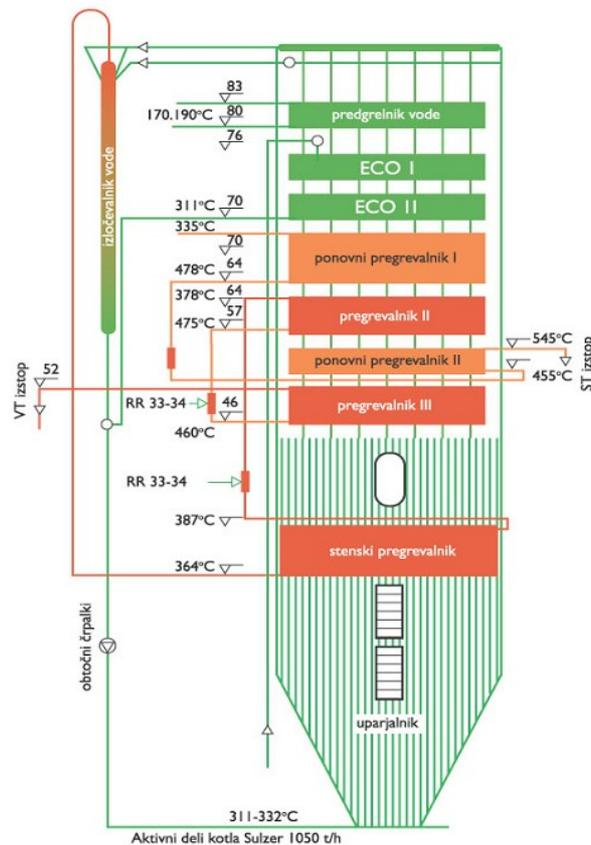
Fig. 1: Schematic of boiler Sulzer, block V. of TE Šoštanj [1].
