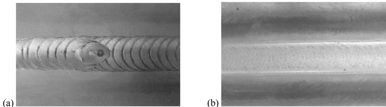
Fig. 3: Appearance of weld root (a) and weld face (b) produced by orbital welding of tube.
