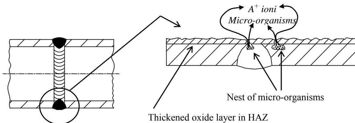
Fig. 1: Pitting corrosion next to weld.
