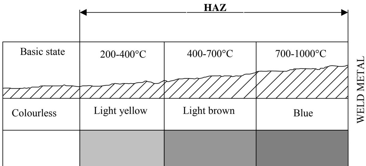
Fig. 2: Thickened oxide film in HAZ gets tinted.
