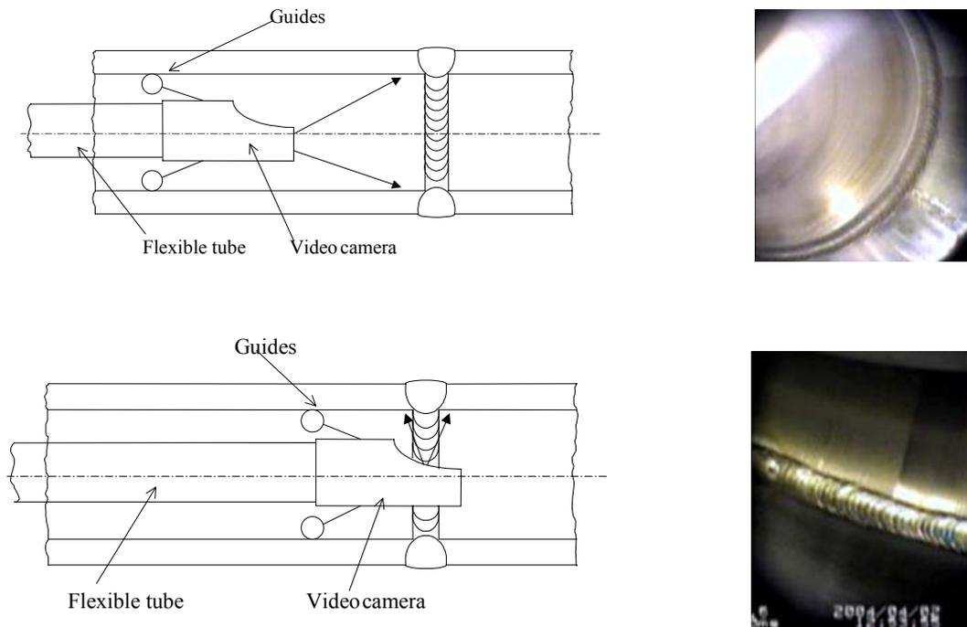
Fig. 5: Views of weld root in direction of tube axis and in direction perpendicular to tube axis.
