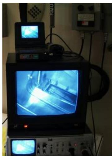
Fig. 6: Camera control unit and a recording device.
