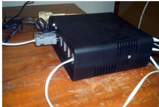
Fig. 4: Image of a measuring logger with connected thermal probes.
