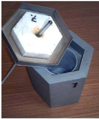
Fig. 3: Images of measuring set of isoperibolic calorimeters for assessment of intensity of hydration heat development.
