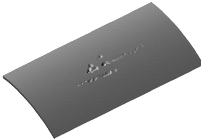
Fig. 2: Solid model of the corroded pipeline segment.
