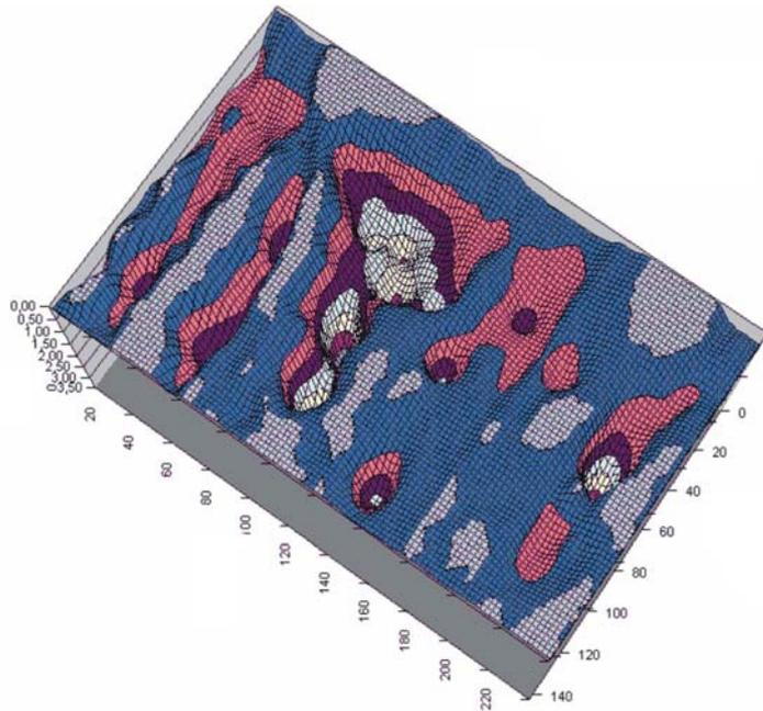
Fig. 1: Geometric shape of gas pipeline wall corrosion defined using ILI data.
