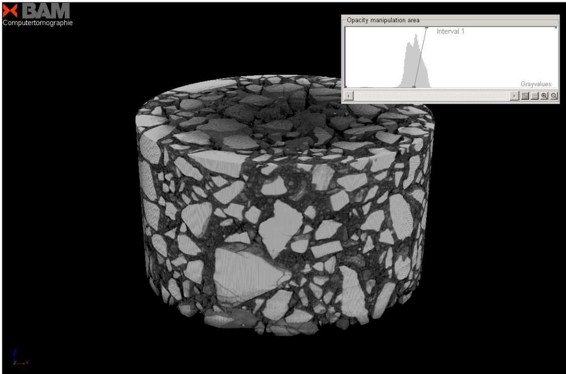
Fig. 3 Surfaces of the same cylindrical drilled concrete sample note the parameter settings
