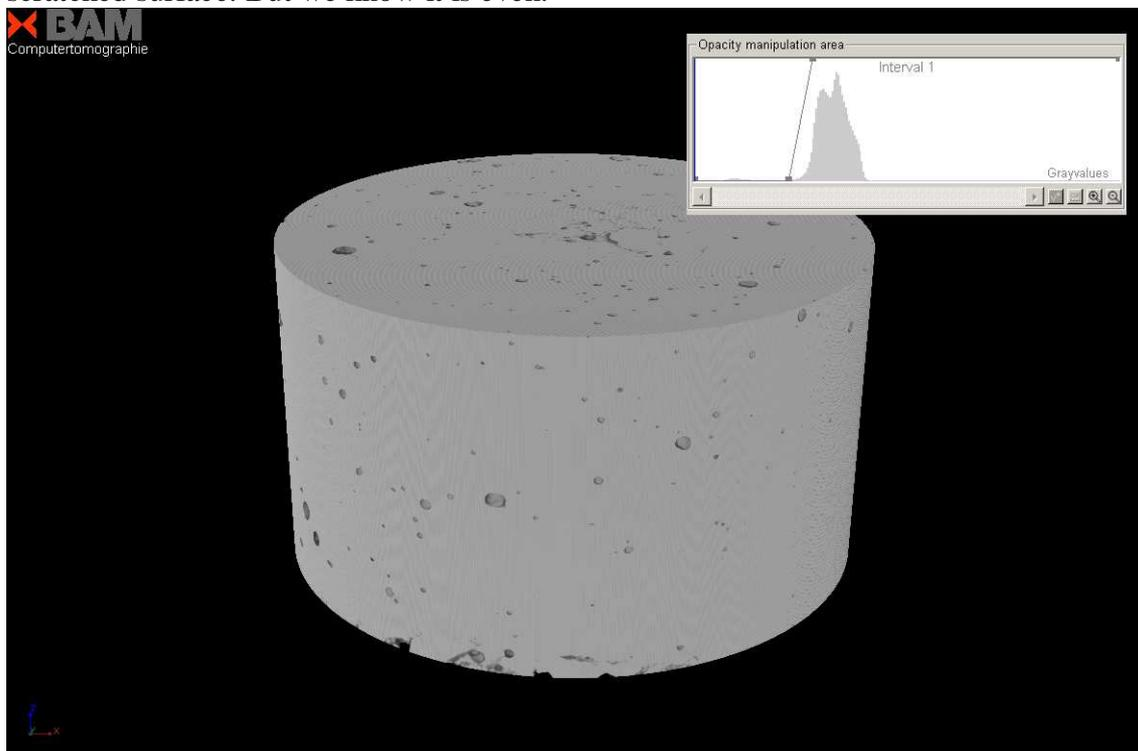
Fig. 2 Surface of a cylindrical drilled concrete sample note the parameter settings.
