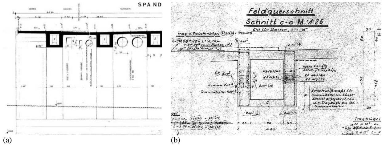
Figure 1: (a) Cross section of the Spandauer-Damm-Brücke consisting of box girders and integrated bridge deck; (b) detail of one box girder with the arrangement of the tendon ducts
