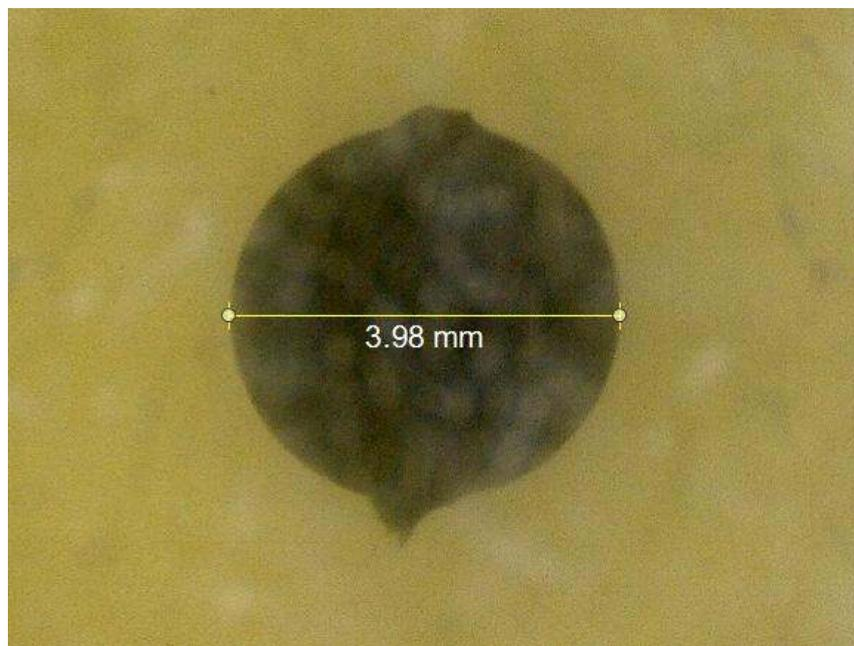
**Figure 2**      **4mm diameter spheres photographed through matrix using microscope**
