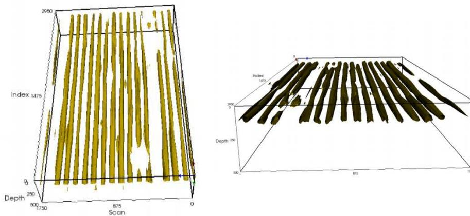
Figure 10 – Top and front view of the slab with the internal hollow cores surface.
