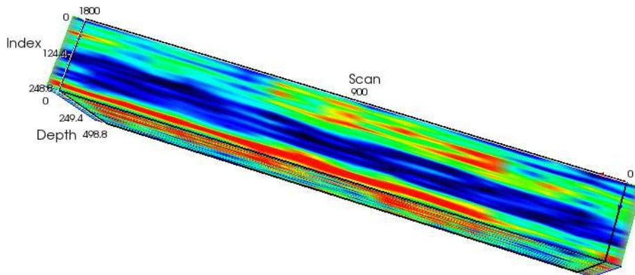
Figure 5 – MIRA results at longitudinal directions.
