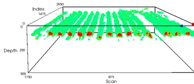
Figure 7 – Identification of hollow cores in sectional, using the 5x10 cm grid.
