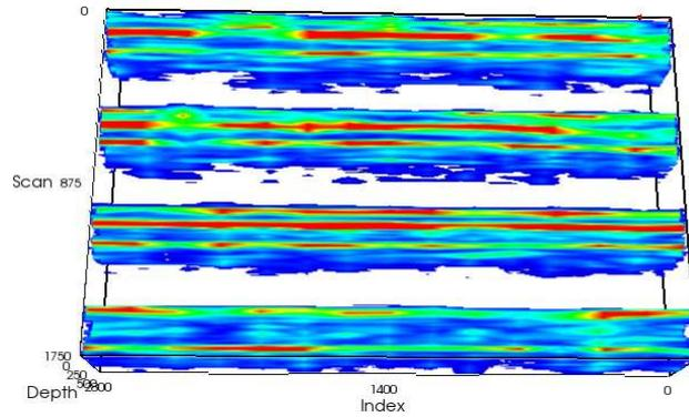
Figure 9 – Results of ultrasonic tomography with 25x50 cm grid.
