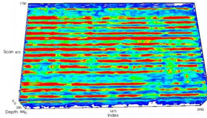
Figure 6 – Results of ultrasonic tomography with 5x10 cm grid.
