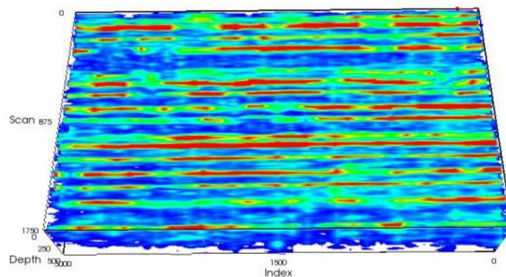
Figure 8 – Results of ultrasonic tomography with 10x25 cm grid.
