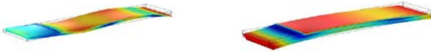
Figure 2: Picture of the numerical mode shape of piezoelement (left) and piezoelement with alumina (right) at 25 kHz. Colours indicate amplitude of displacements.
