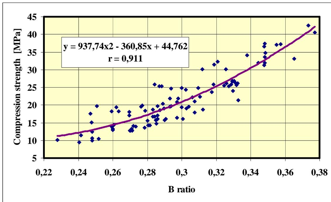
Figure 3. Test Results for “old” solid bricks: relation between  $B$  ratio and compression strength
