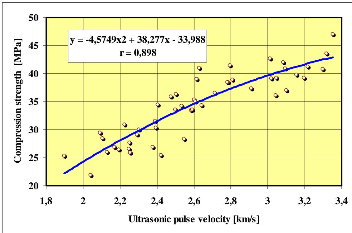
Figure 7. Test results (Liptovsky Mikulas solid bricks) – correlation between ultrasonic pulse velocity and compression strength
