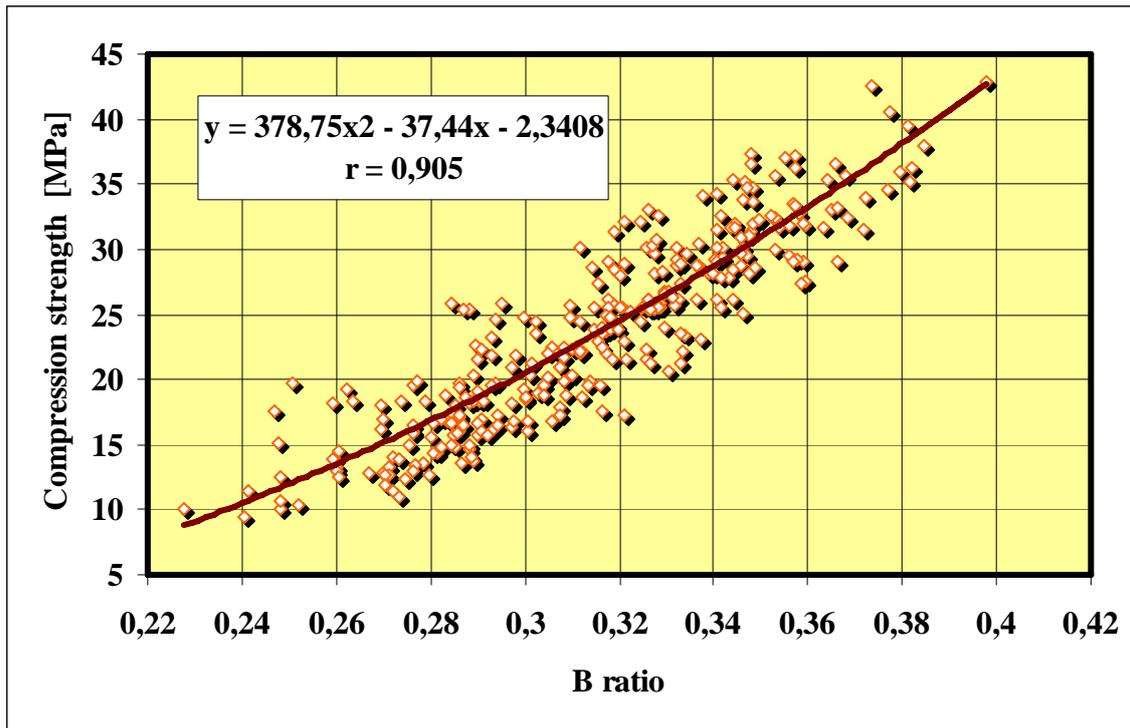
Figure 4. Test Results for solid bricks: – set of 303 test samples (both “old” and “new”)
