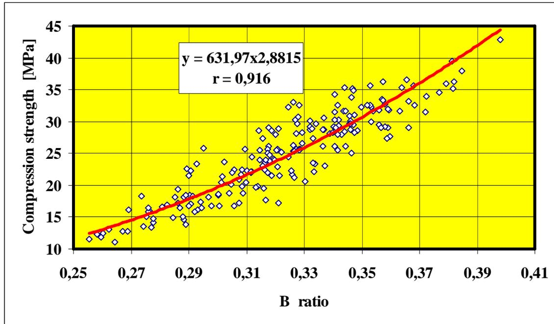
Figure 2. Test Results for “new” solid bricks: relation between  $B$  ratio and compression strength
