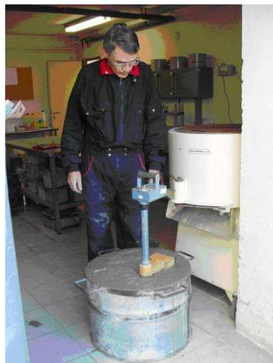
**Figure 8. The radiation density gauge calibration**
