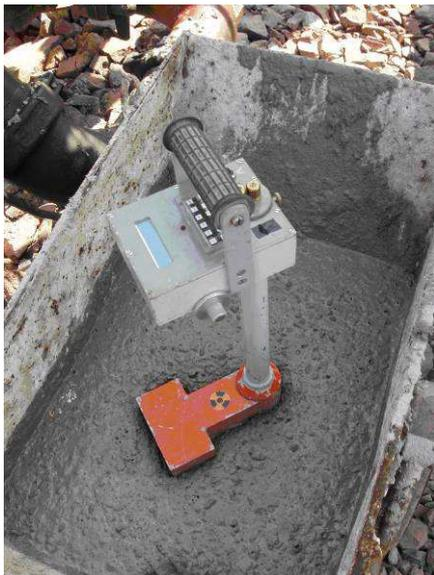
**Figure 4. The concrete mixture testing before placing to formwork**
