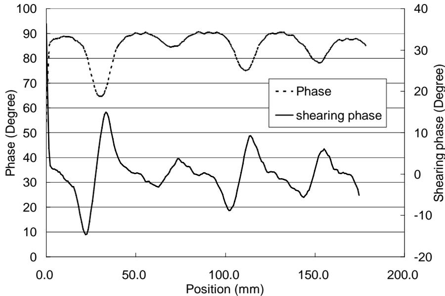
**Figure 5. Thermal Phase and shearing phase distribution at 0.01 Hz of  $\phi$  12 mm**
