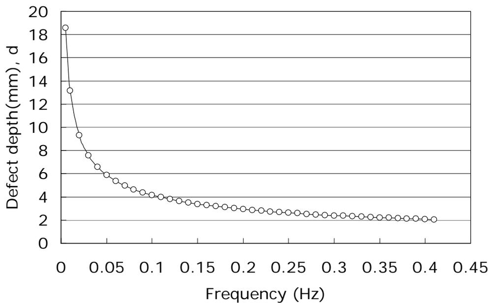
**Figure 4. Detectable defect depth diagram according to induced frequency**
