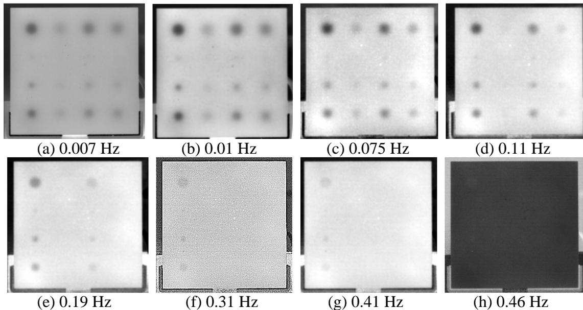
**Figure 3. Thermal phase images of reference specimen at each induced heat source**
