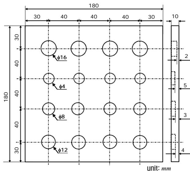
**Figure 2. Reference specimen for lock-in photo-infrared thermography**
