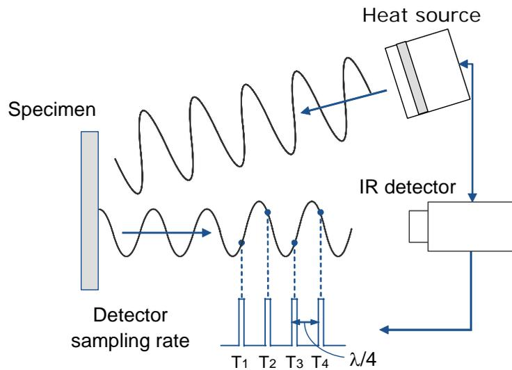
**Figure 1. System configuration and signal processing of lock-in thermography**
