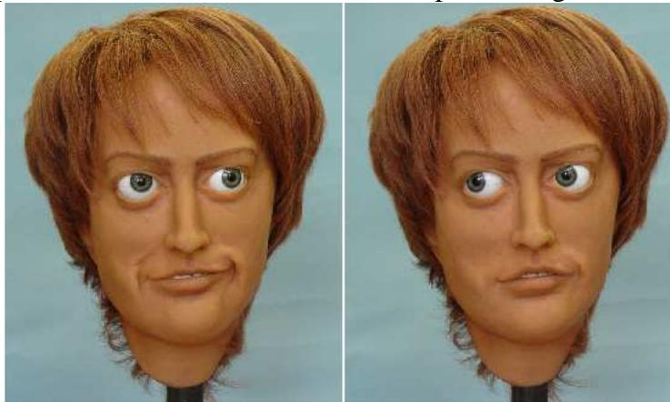
**FIGURE 4:** An android head (Photographed at JPL) making facial expressions. This head is available at JPL as a testbed for EAP actuators. [Courtesy of D. Hanson, Hanson Robotics, LLC]
