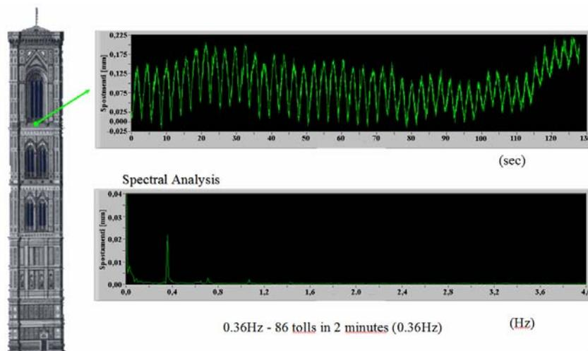
Figure 4: Measured displacement of Giotto's tower
