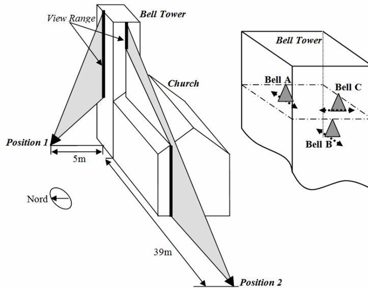
**Figure 10: geometry of measurement of Pratolino's bell tower**
