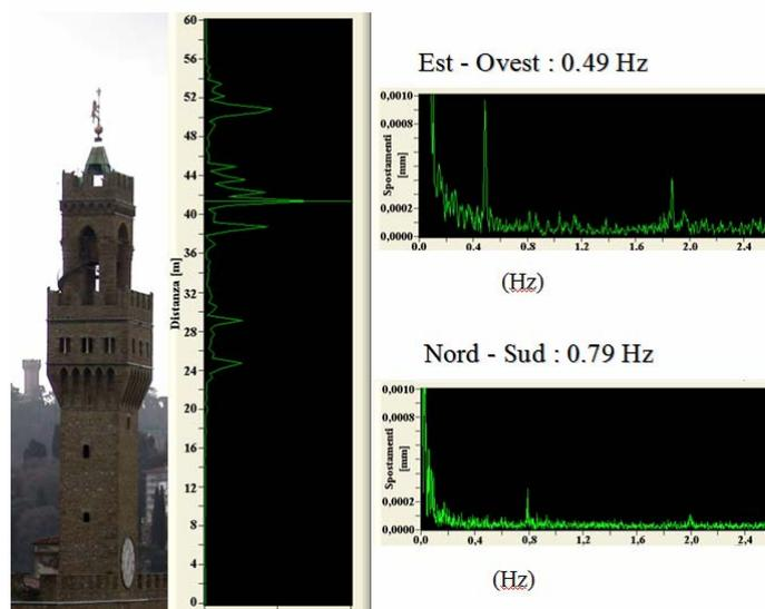
Figure 5: Radar image and measured natural frequencies
