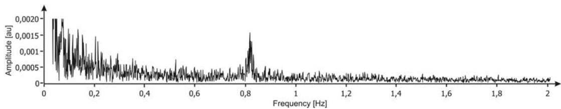
**Figure 8: FFT of phase signal of the pixel corresponding to Arnolfo's Tower**
