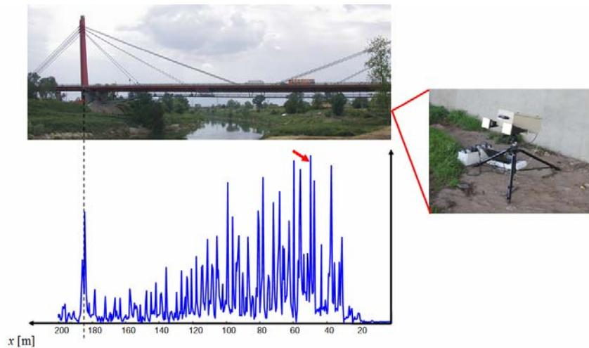
Figure 12: testing and radar image of the Indiano's bridge
