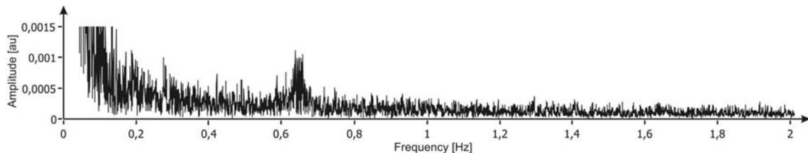
**Figure 9: FFT of phase signal of the pixel corresponding to Giotto's Bell Tower**
