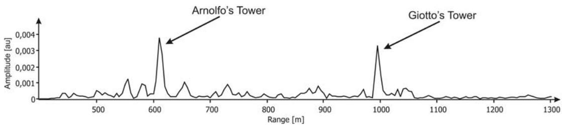
**Figure 7: Radar range profile with two peaks of Arnolfo's Tower and Giotto's Tower**
