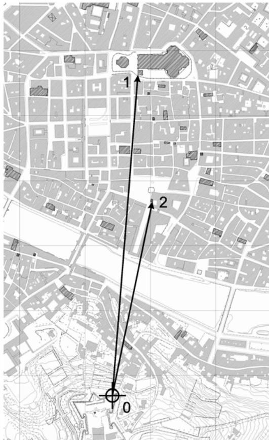
**Figure 6: Map of Florence including the arrangement of the measure: 0 is the radar position; 1 is the Giotto’s Bell Tower position; 2 is the Arnolfo’s Tower position.**
