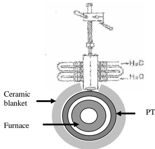
**Fig.1. Device to form hydride blisters by thermal gradient.**
