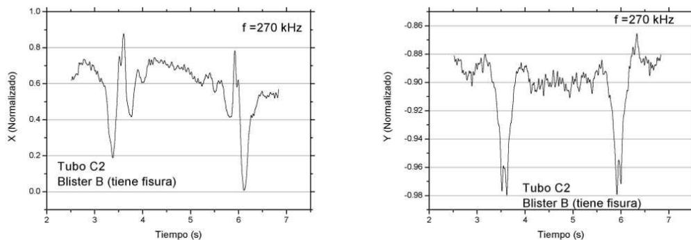
**Fig .3. Eddy currents X(T) Y(t) signals for blister b in C2**
