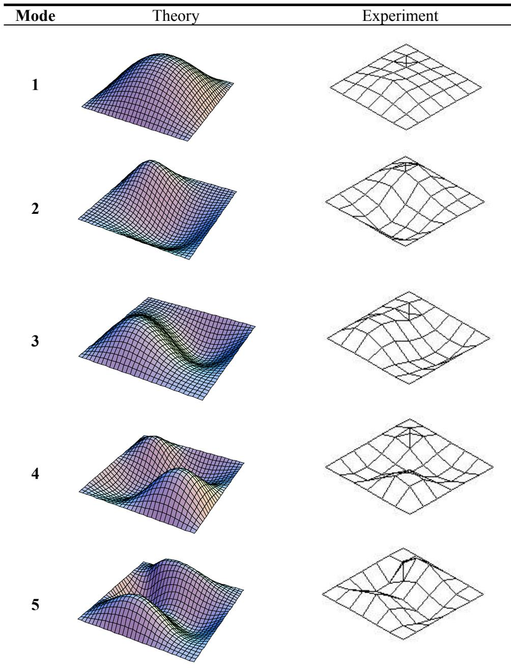
**Figure 8. Theoretical and experimentally LDV-detected first 5 mode shapes of a 4-side constrained steel plate.**
