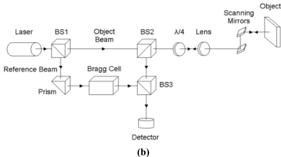
**Figure 3. (a) Schematic view of scanning laser vibrometry; (b) the Polytec laser Doppler vibrometer at the laboratory of the University of Parma.**
