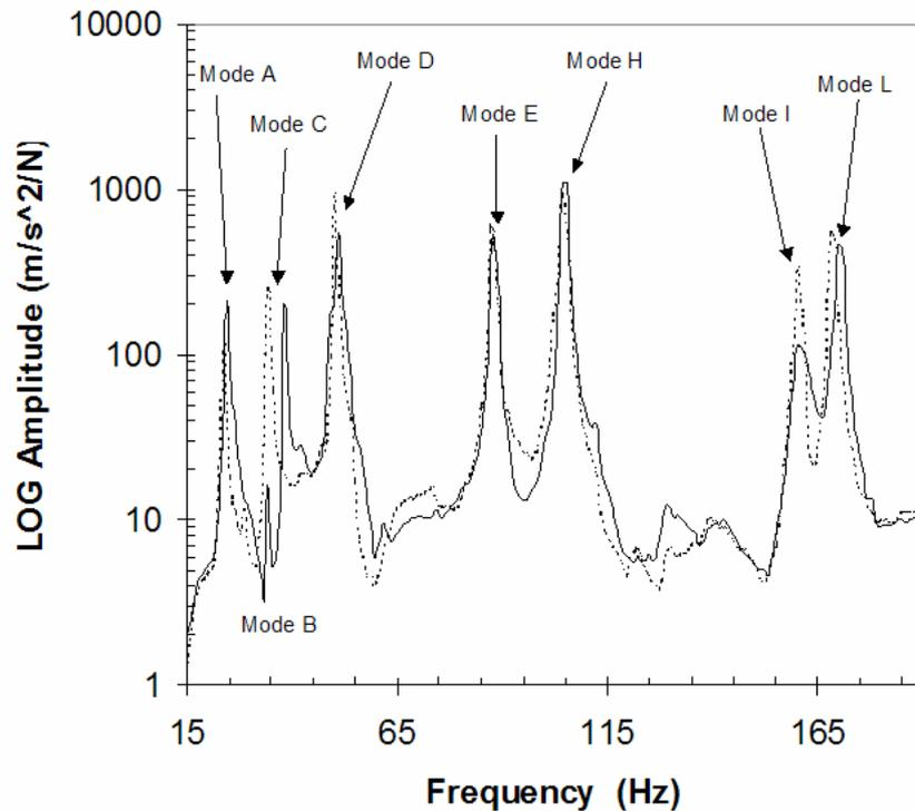
**Figure 9. Comparison between the theoretical (dot line) and the experimental (solid line) dynamic response of a square plate.**
