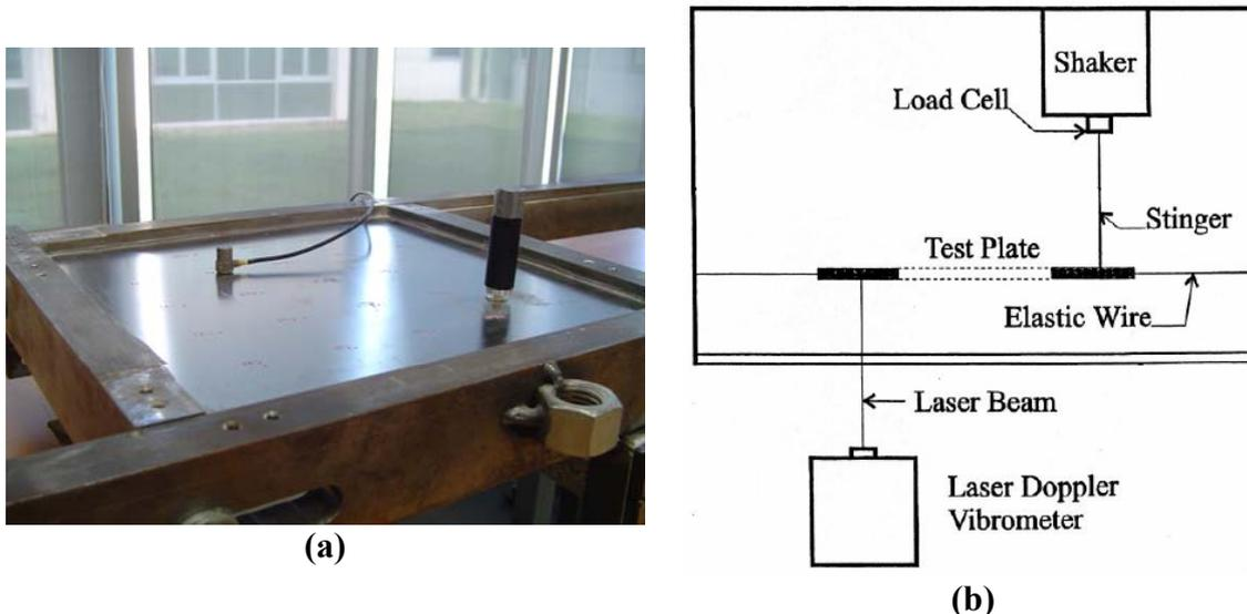
**Figure 6. (a) The 4-side constrained steel plate for the validation of the laser Doppler measurement method; (b) Diagram of the experimental set-up.**
