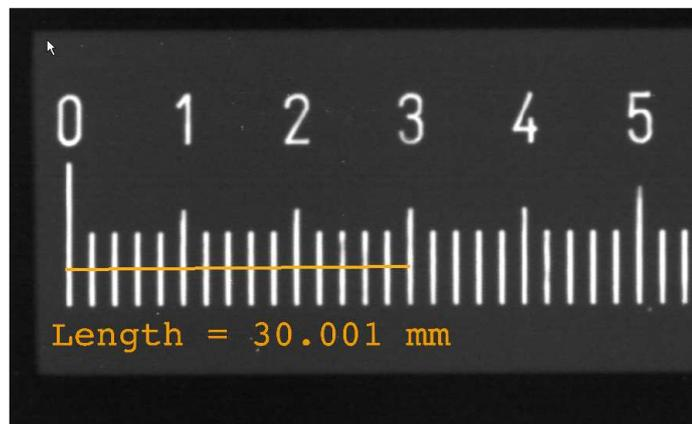
**Figure 9. Example of a measurement at one end of the IP using the phantom's metric ruler**
