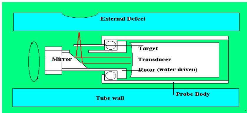
**Figure 2. Probe assembly**
