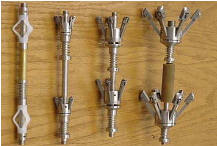
**Figure 16. Centering devices up to 75 mm diameter**
