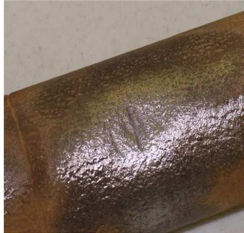
**Figure 9. Internal Dent**
