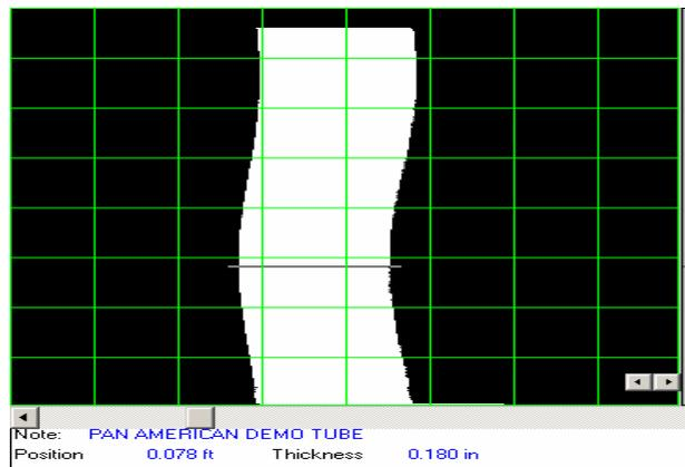
**Figure 4. B Scan image of the tube**
