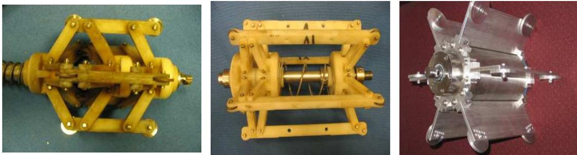
**Figure 17. Centering devices for diameters up to 300 mm**
