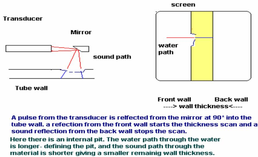
Figure 5. Internal defects measurement
