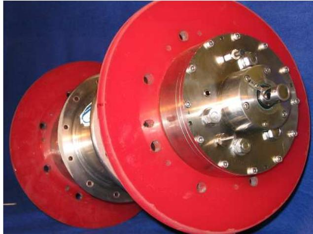
**Figure 18. Centering devices for 250 mm – 1100 mm diameters pipelines**
