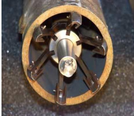
**Figure 1. Turbine and centering device**
