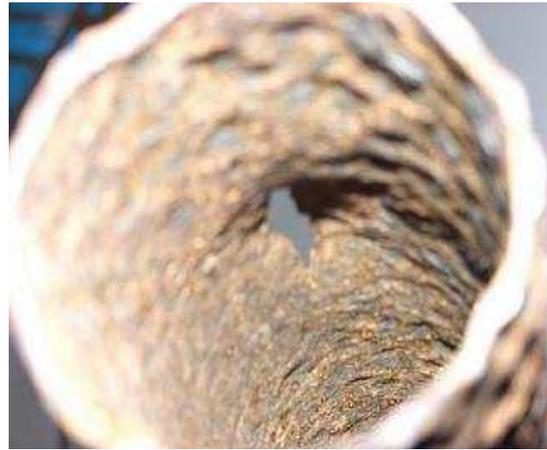
**Figure 12. Corroded tube**
