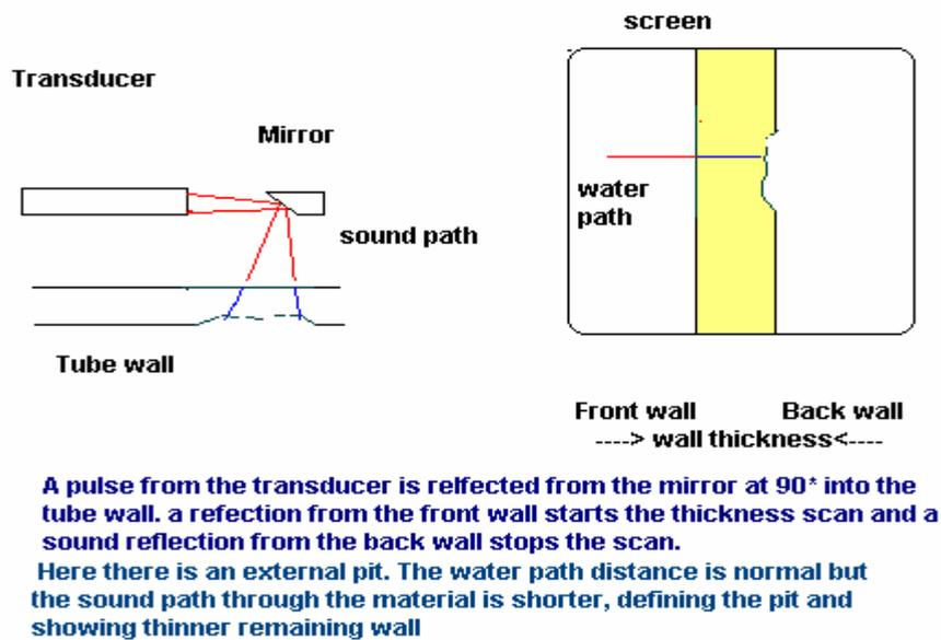
Figure 6. External defect measurement
