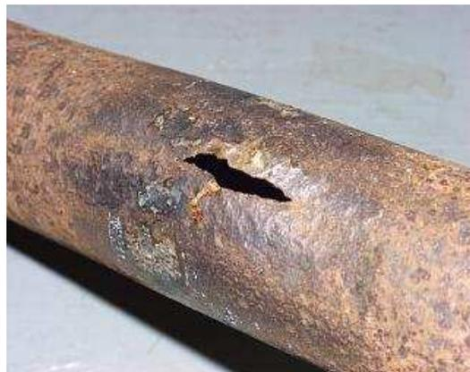
**Figure 11. Expanded, split tube**
