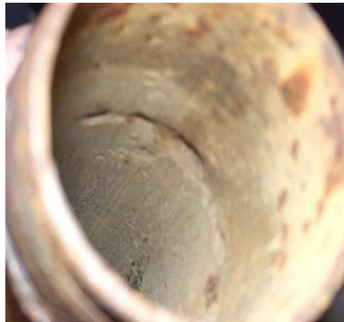
**Figure 10. Severe internal corrosion area**
