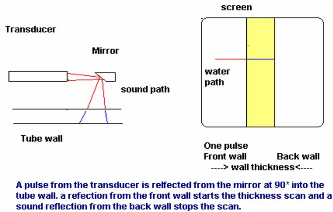
**Figure 3. Thickness measurement principle**
