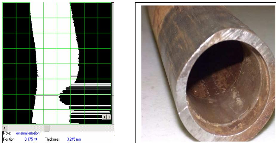
Figure 8. External erosion
