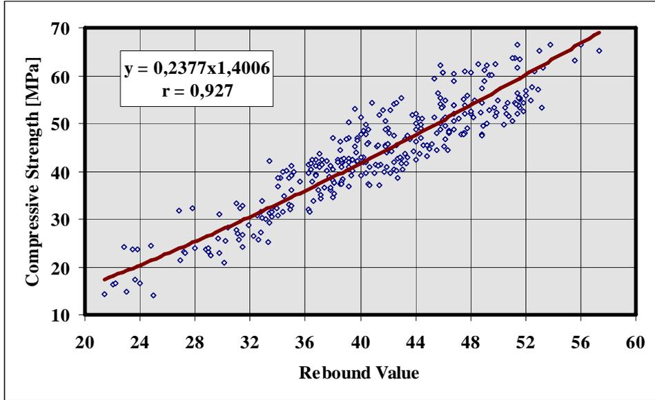
**Figure 4. GFC-C Test Results, Dependency on Relation between N-Type of Schmidt Hammer Rebound Value and Compression Strength**
