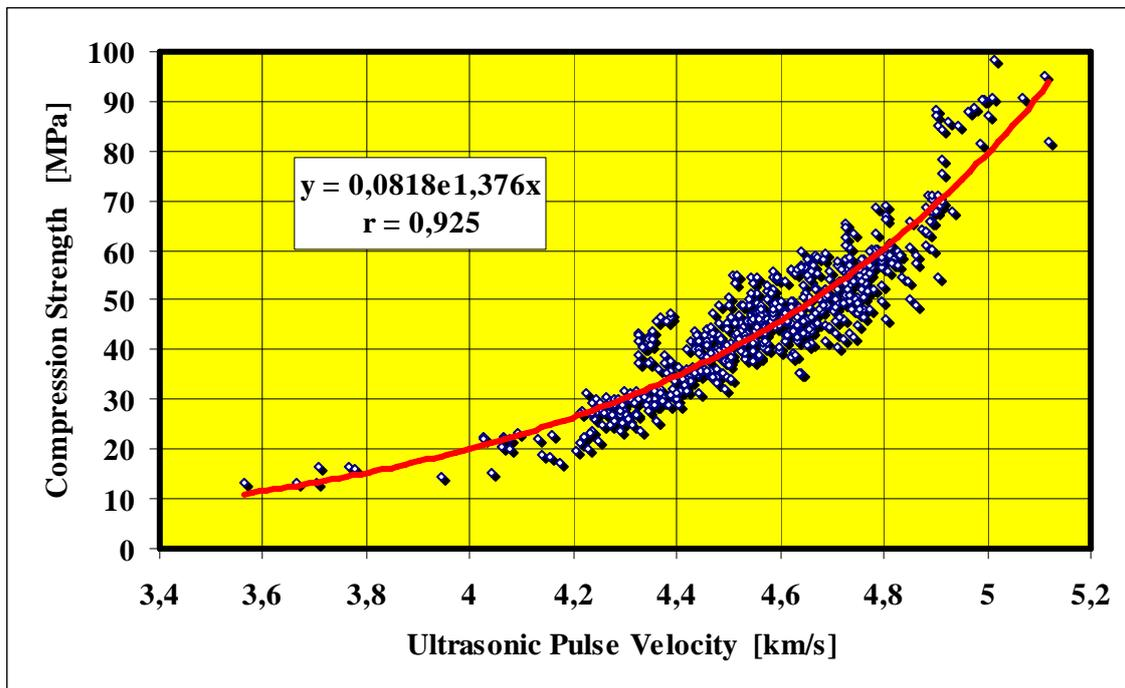
**Figure 2. Test Results. Measuring of Relations Depending on Ultrasonic Pulse Velocity and Compression Strength on Gypsum Free Cements**
