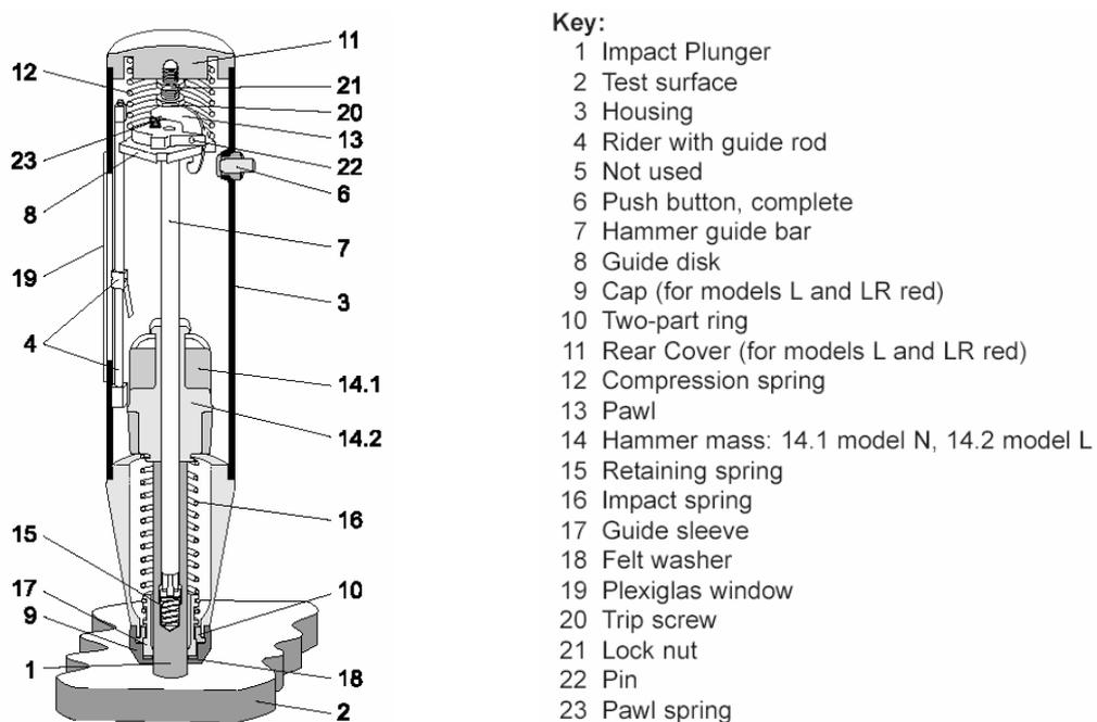
**Figure 3. Description of Concrete Test Hammer Schmidt, Types N / L (source: [www.proceq.com](http://www.proceq.com))**
