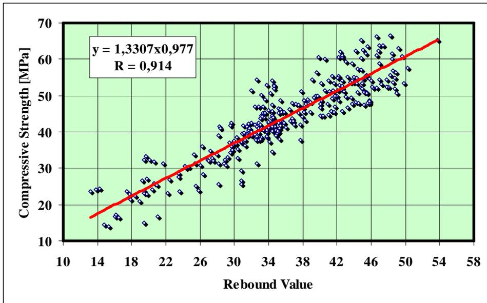
**Figure 5. GFC-C Test Results, Dependency on Relation between L-Type of Schmidt Hammer Rebound Value and Compression Strength**
