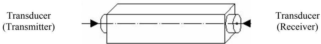
**Figure 1. Scheme of Direct Transmission**
