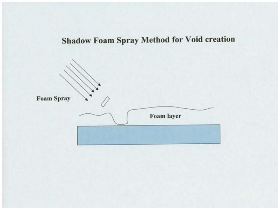
**Figure 2. Shadow Method for Natural void creation**
