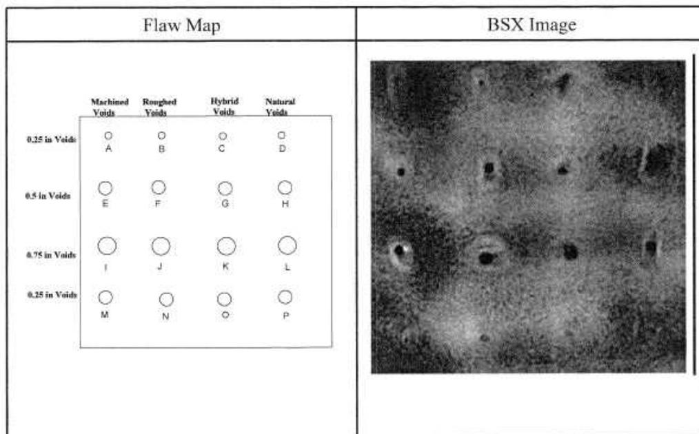
**Figure 5. Flaw map and BSX Image of panel comparing machined, roughed, hybrid and natural flaws.**
