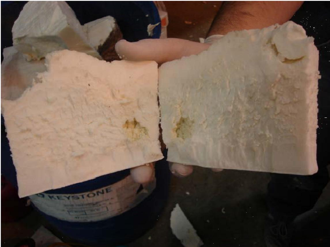
Figure 1. Example of a naturally occurring void.
