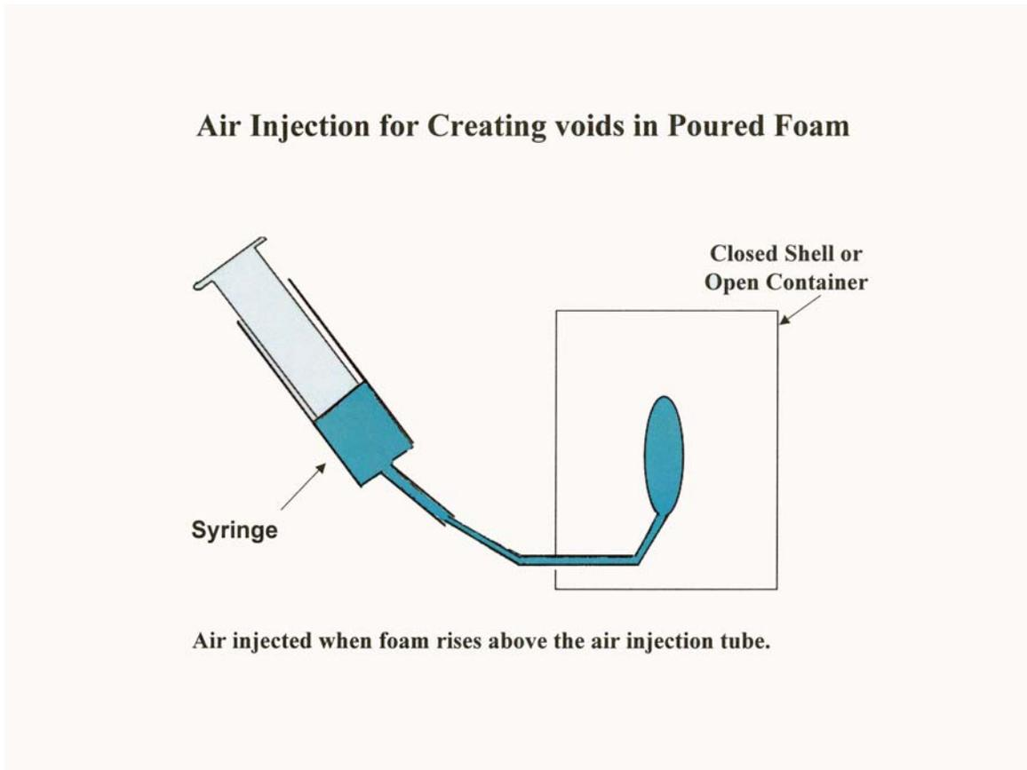
**Figure 3. Air injection Method for Natural Void creation**
