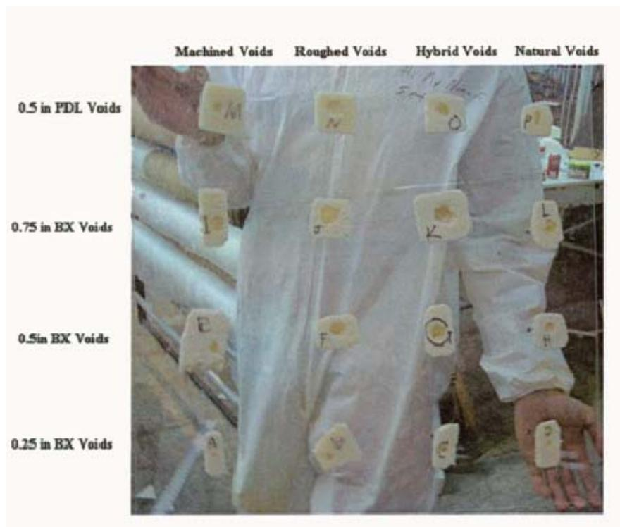
**Figure 6. Plexiglass Panel with multiple flaws inserts**
