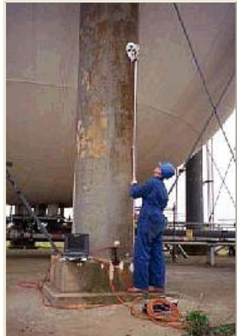
Fig 5: Application on concrete covered object: support legs of spherical storage tanks.
