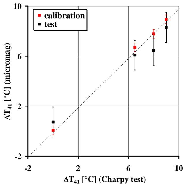
**Figure 5. Prediction of the shift of the ductile-to-brittle transition temperature by the micromagnetic method**
