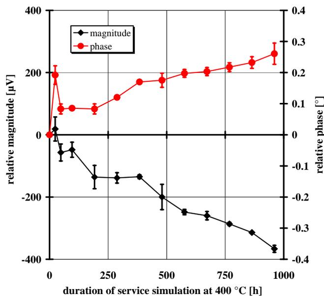
**Figure 1. Eddy current quantities magnitude and phase as a function of service exposure duration for initially recovery-annealed (3 h / 600 °C) WB 36 steel**
