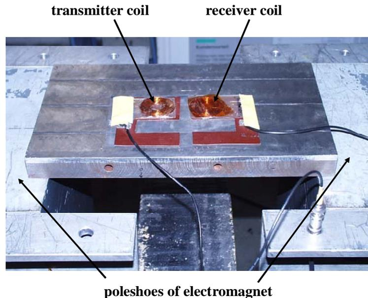
**Figure 6. EMAT configuration with HF-coils and laboratory electromagnet**
