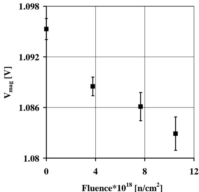
**Figure 3. Correlation between the eddy current impedance magnitude and the neutron flow**
