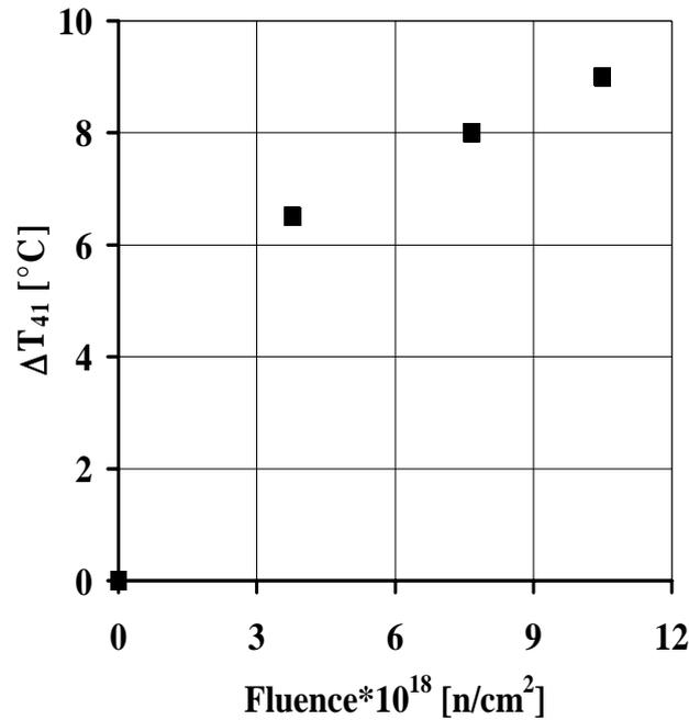
**Figure 4. Dependency of the ductile-to-brittle transition temperature on the neutron flow**
