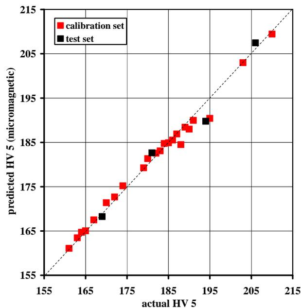
**Figure 2. Predicted Vickers hardness for WB 36 versus actual Vickers hardness**
