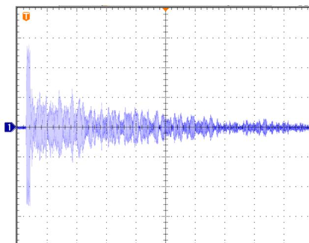
**Figure 8. Ultrasound signals generated by an excitation through a PVC plate (8 mm thickness), magnetic field strength: 260 A/cm, frequency: 50 kHz**
