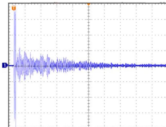
**Figure 7. Ultrasound signals by an excitation on the austenitic clad side (8 mm thickness), magnetic field strength: 260 A/cm, frequency: 50 kHz**
