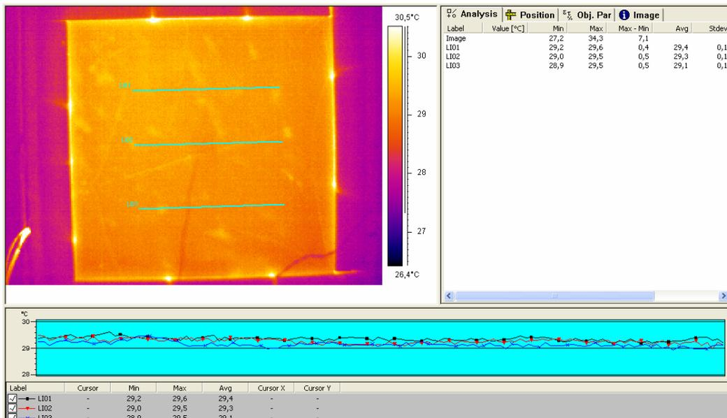
**Figure 6. Thermogram of sample surface, side A
