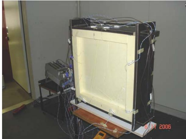
**Figure 3. The test rig for prefabricated panel**
