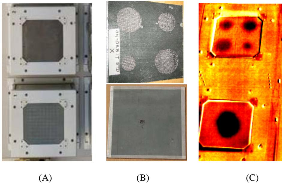
**Figure 10. (A) Photograph of the OML surface of the two RCC samples in the Shuttle cargo bay. No OML surface damage is visible on either sample. (B) Photographs of the IML surface of the same two samples. (C) Processed infrared NDE imagery from STS-121 flight test.**
