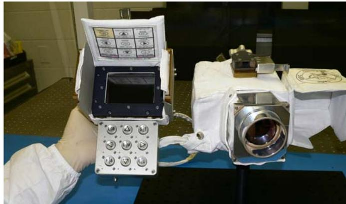
**Figure 1. Photograph of EVA IR Camera Flight Unit. The camera consists of two major components: the camera body with the germanium infrared detector, battery, memory, and flash drive, and the Remote Control Unit (RCU) containing the LCD screen and control buttons.**
