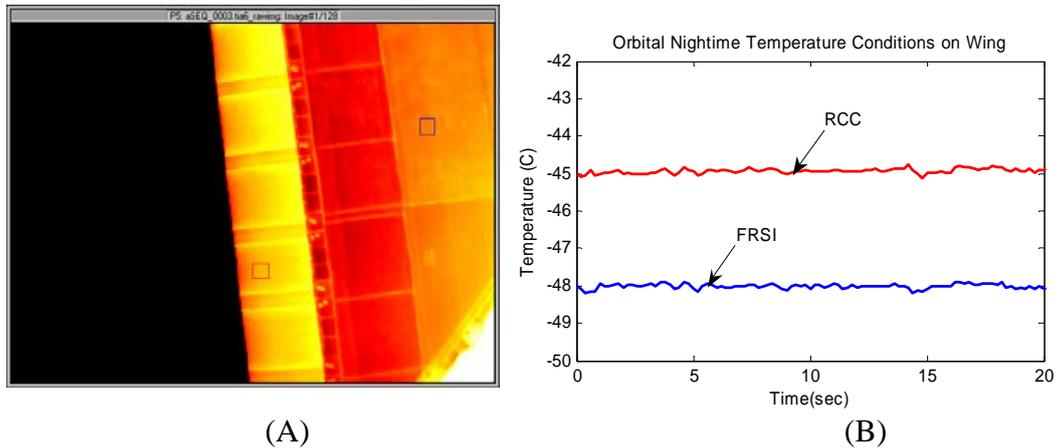
**Figure 9. (A) Infrared image from Shuttle wing leading edge taken at 07:16 CDT on July 15, 2006. Orbital sunrise will occur in approximately 5 minutes. (B) Temperature versus time plots for two regions of the infrared image.**
