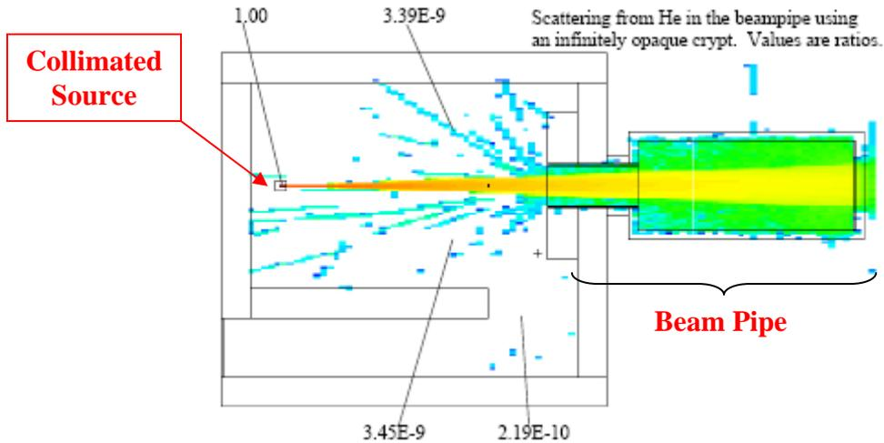
**Figure 5. A well-collimated system impacting on a beam pipe. Note that only a minimal amount of radiation (light blue and green traces occurring at various angles to the central [yellow] beam) escapes back into the room.**
