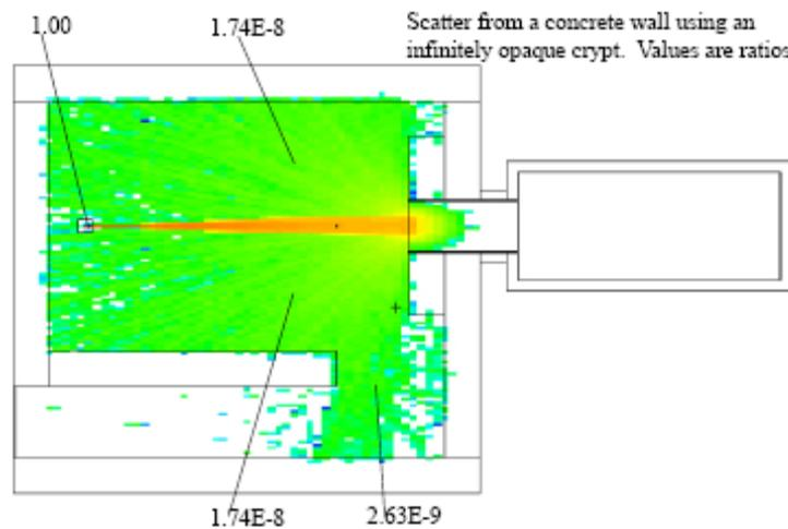
**Figure 6. Blocking the beam pipe, or equivalently not using a beam pipe behind the object being imaged, results in significant scatter that essentially fills the radiography bay.**
