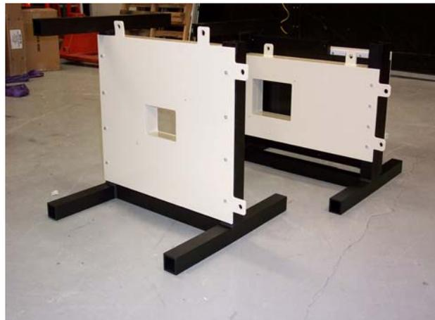
**Figure 3. A series of square holes of decreasing size used to reduce beam scatter.**
