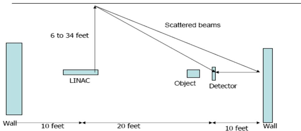
**Figure 1. Simulation geometry.**
