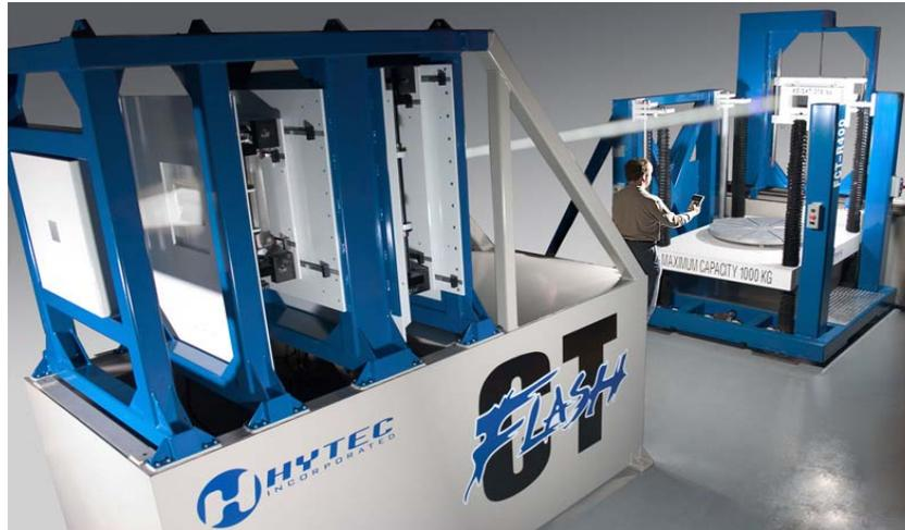
**Figure 4. A complete radiography system with pre- and post-collimators. The collimator next to the detector masks the detector, effectively shielding it from scattered photons.**
