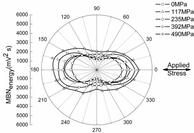
**Figure 3. Polar plots of  $MBN_{energy}$  for sample oriented along the Rolling Direction at different stress value**
