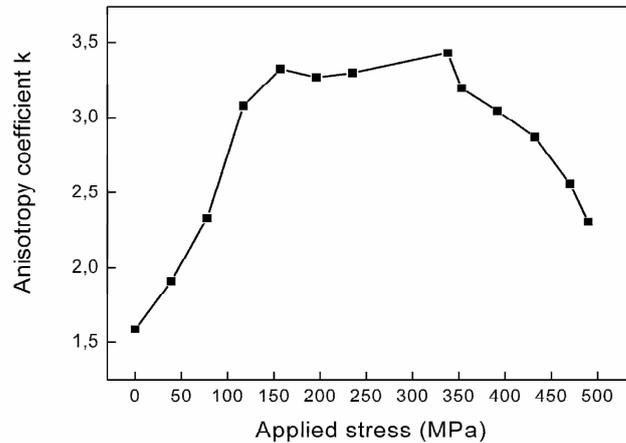
**Fig. 5** Dependency of coefficient de anisotropic with applied stress
