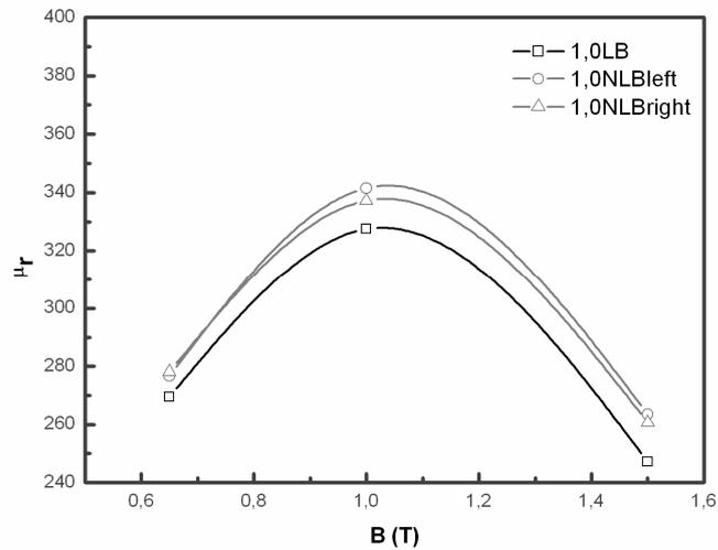
**Figure 6. Relative Permeability of the 1% deformation in the R D sample.**
