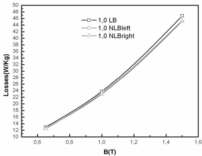
**Figure 7. Losses of the 1% deformation in the R D sample.**
