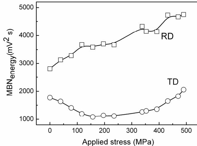
**Figure 4. Dependence of the MBN energy on the applied stress, for rolling (RD) and transversal (TD) directions**
