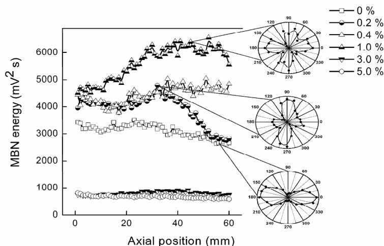
**Figure 2.  $MBN_{energy}$  variation over the half-gauge zone for different strains in the Rolling Direction sample.**
