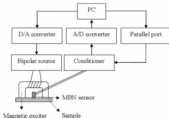
**Figure 1. Experimental setup for measurement of the MBN signal.**
