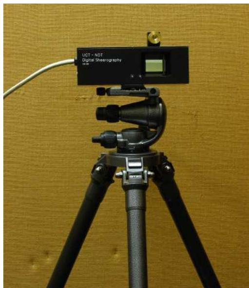
Figure 2. Portable Digital Shearography prototype
