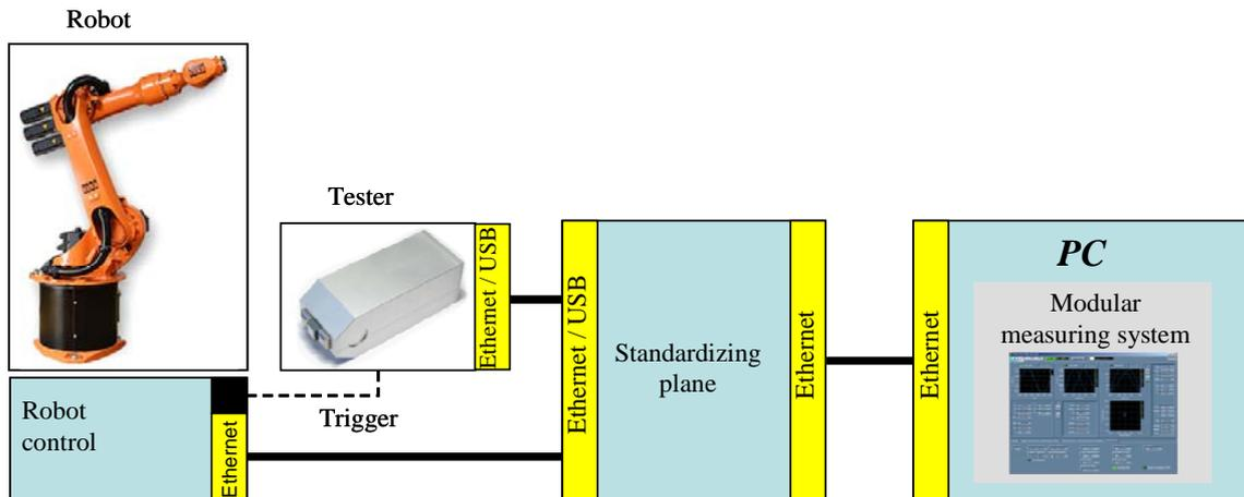
**Figure 8. Modular Robotic Platform w/ Standardized Control Module**
