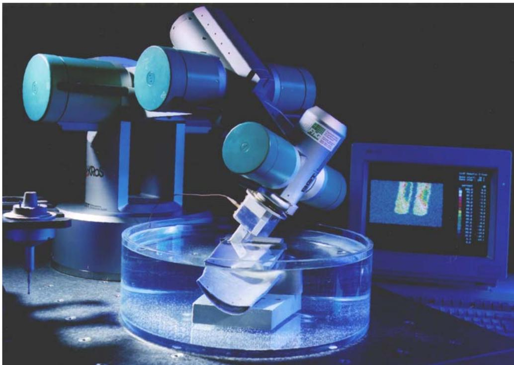
**Figure 9. Ultrasonic Inspection of Freeform Surface Objects**
