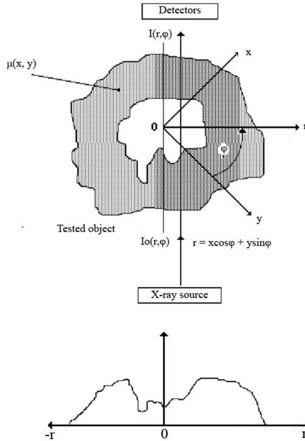
**Figure 1. The X-ray passing through the object and definition of coordinates**
