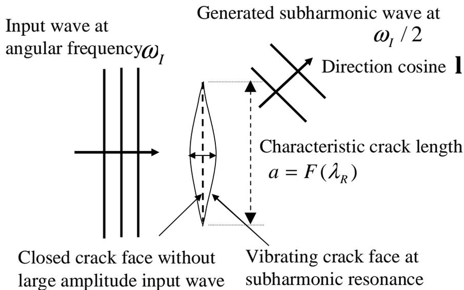
**Figure 1. Subharmonic resonance at a closed crack**
