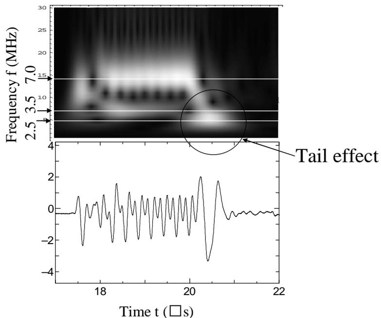
**Figure 4. Wavelet transform of subharmonic wave and tail effect in transmission configuration**
