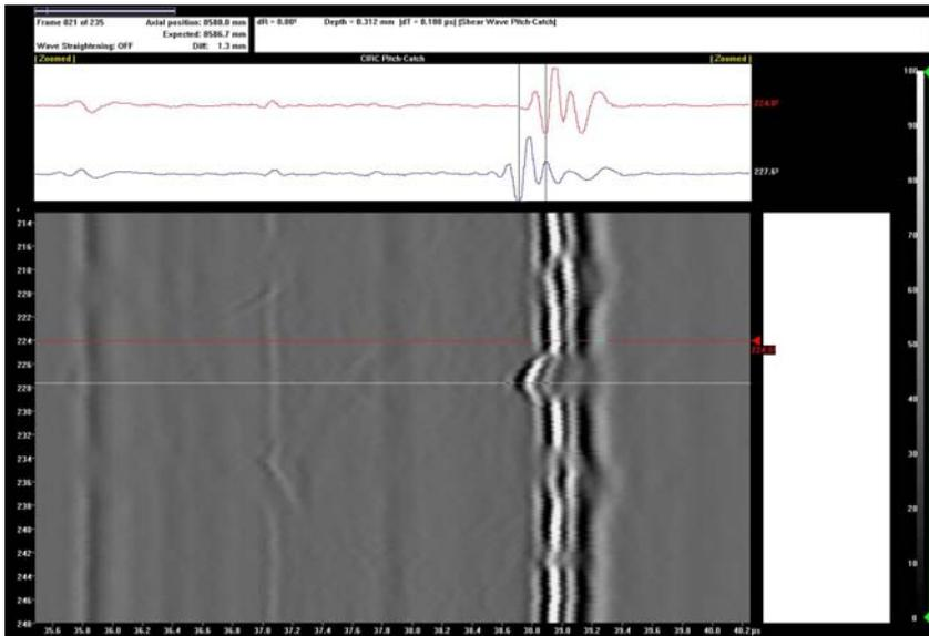
Figure 6 Sizing of flaw using Pitch Catch B-scan
