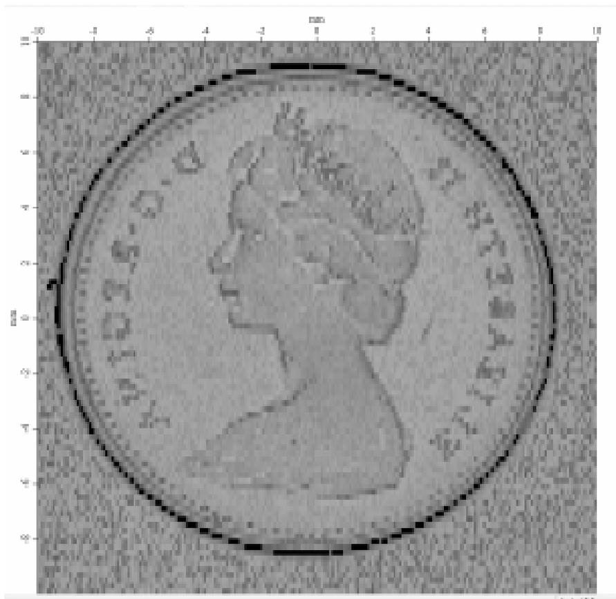
Figure 4 10 cent coin (Canadian) scanned in water using 20 MHz probe. Image reversed.
