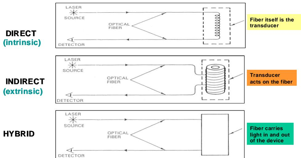
**Figure 3. Classification of optical fiber sensors**
