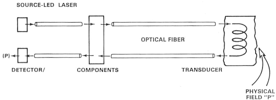
**Figure 2. Basic elements of an optical fiber sensor**
