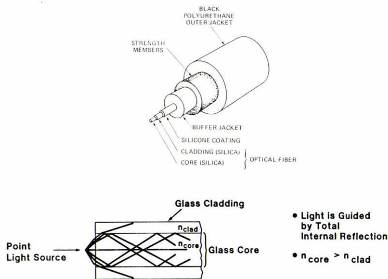
Figure 1. Schematic of an optical fiber
