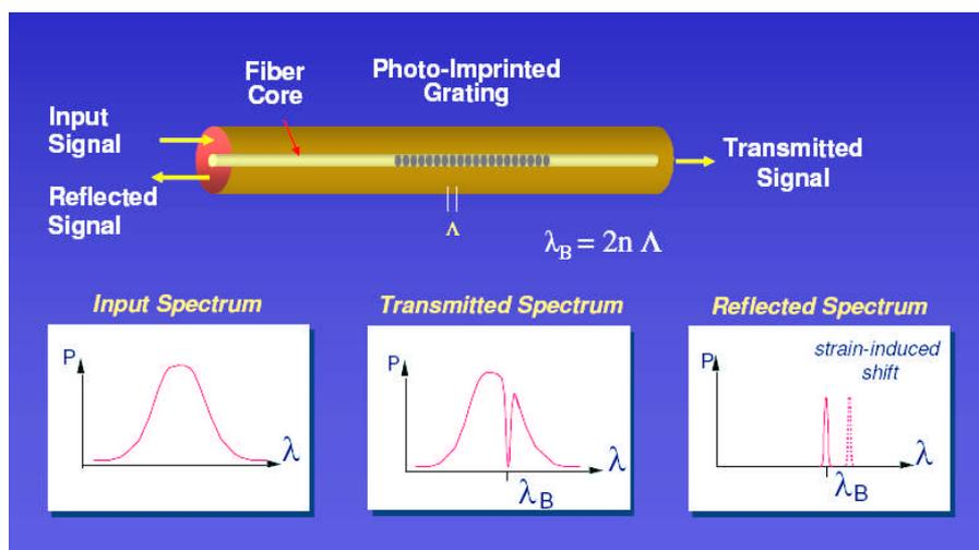
**Figure 4. Transmission and reflection spectra of a fiber Bragg grating**
