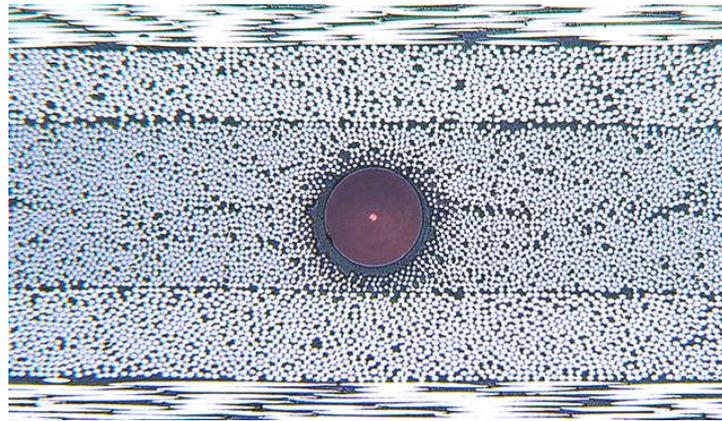
**Figure 7. Carbon Fiber Reinforced Polymer Composite with embedded fiber optic Bragg grating sensor (source; Daimler-Benz).**
