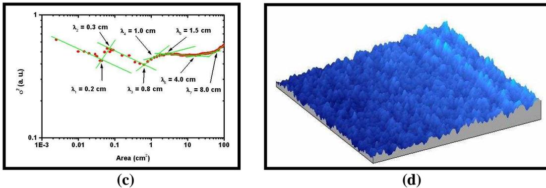
Figure 5. Symmetric sample plate study. (a) Digitized image of the plate. (b) RIMAPS analysis. (c) Variogram results. (d) 3D representation of the surface using a cut-off length of 3 mm.
