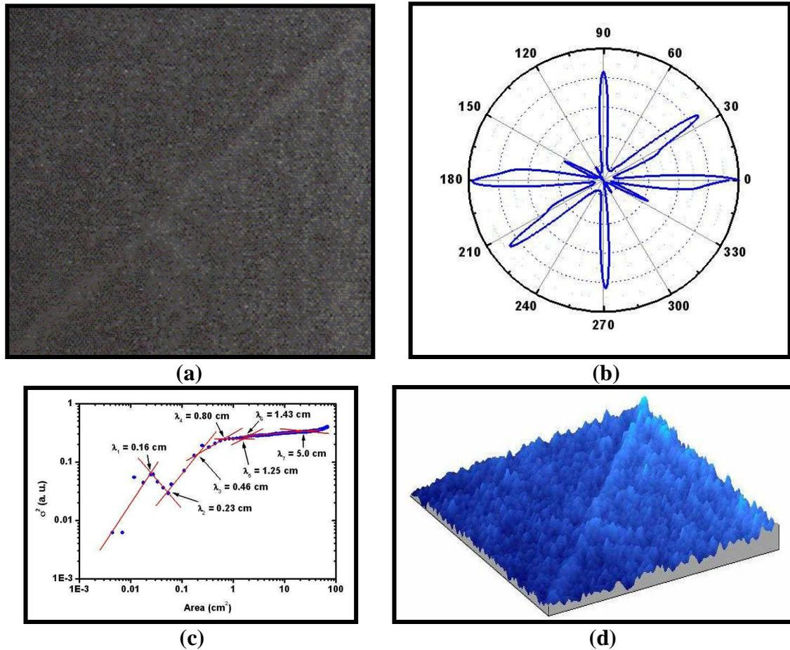
Figure 7. Symmetric and overlapped sample plate study. (a) Digitized image of the plate. (b) RIMAPS analysis. (c) Variogram results. (d) 3D representation of the surface using a cut-off length of 2.3 mm.
