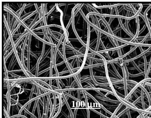
**Figure 3. SEM image of the bleeder.**
