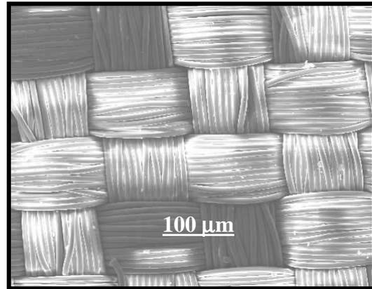
**Figure 2. SEM micrograph of peel ply surface.**
