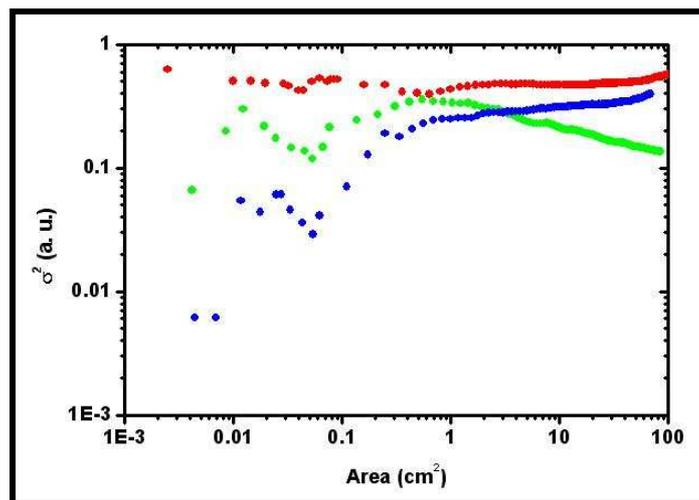
Figure 8. Comparison of Variogram results. The three cases represented are: ● symmetric laminate, ● non-symmetric laminate, ● symmetric laminate with overlapping of fibres. The distribution of data varies when a defect is introduced in the manufacturing process.
