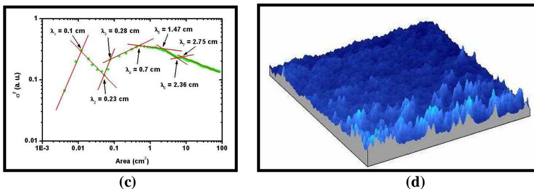
Figure 6. Non-symmetric sample plate study. (a) Digitized image of the plate. (b) RIMAPS analysis. (c) Variogram results. (d) 3D representation of the surface using a cut-off length of 2.8 mm.
