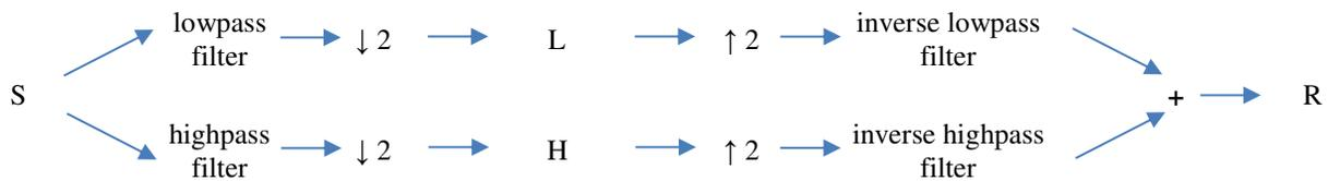
**Fig. 2** Transforming a one-dimensional signal  $S$  into its lowpass ( $L$ ) and highpass ( $H$ ) components and backwards ( $R$ ).
