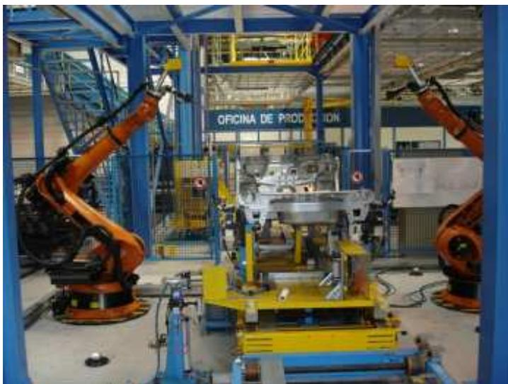
Figure 9: General view of a production CYCLOPS system using dual robotic test heads
