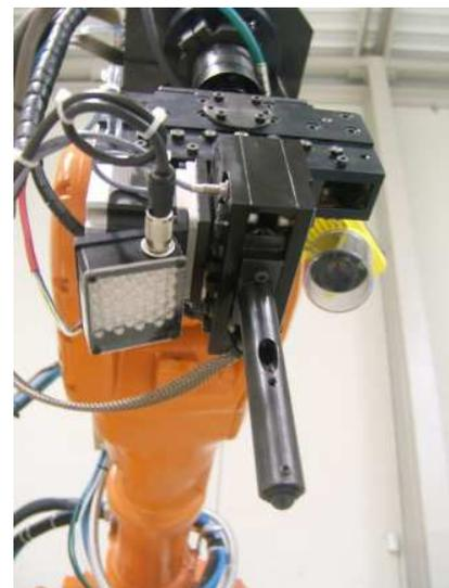
Figure 10: CYCLOPS test head showing machine vision system and probe manipulator
