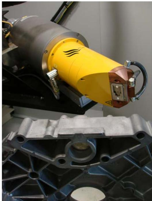
**Figure 4.** A directional microfocus tube examining a large casting. The cooled reflection target allows for higher energy X-rays to be generated.
