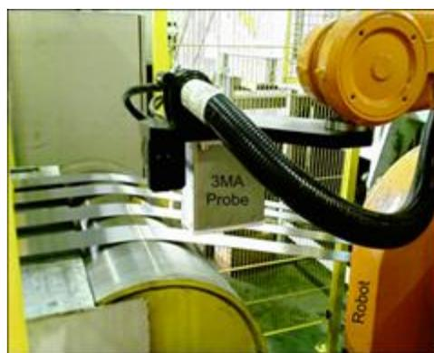
Figure 3. 3MA probe with robot at a strip line
