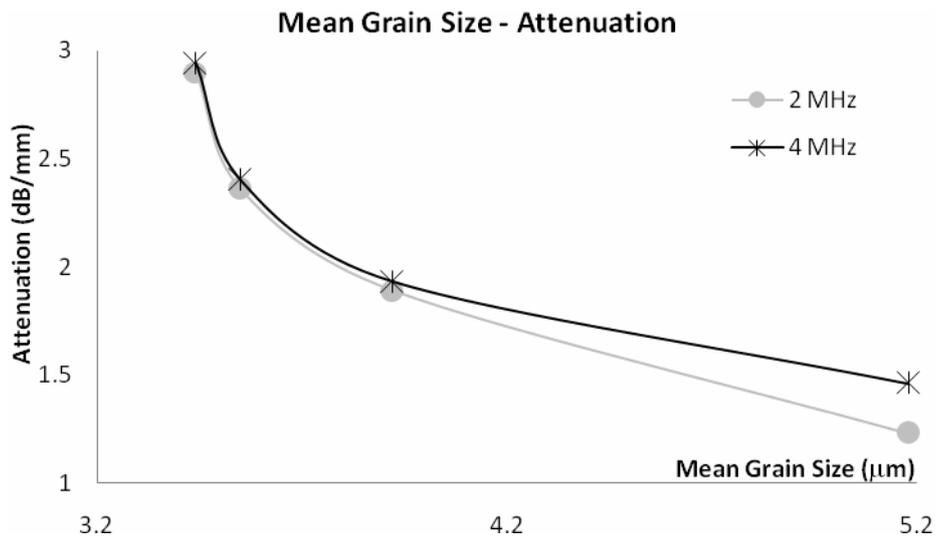
Fig. 2. Attenuation-Mean Grain Size Graph
