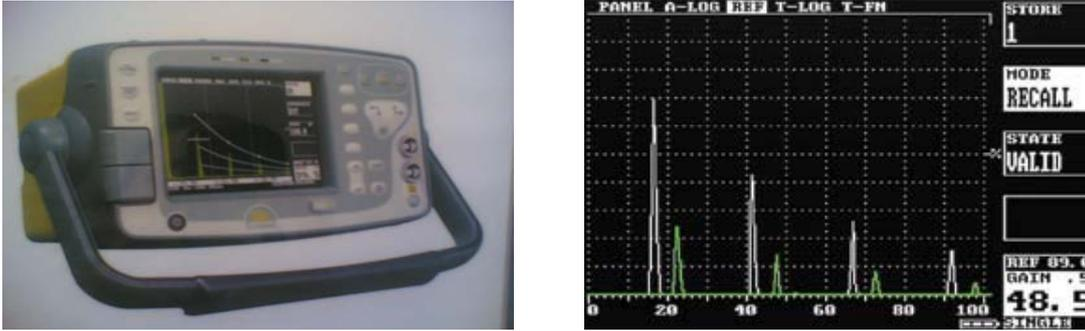
Fig. 1. Flaw detector, front and backwall echoes on screen.
