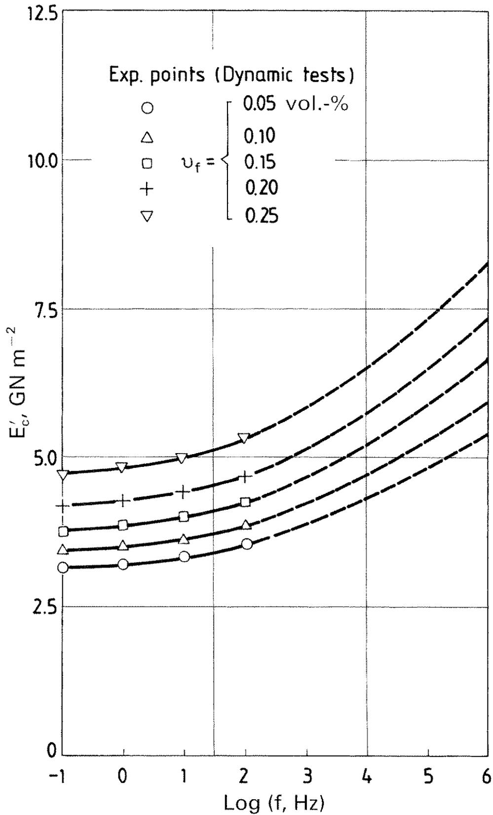
7 Variation of dynamic storage modulus of composite  $E'_c$  versus frequency for different values of filler volume fraction
