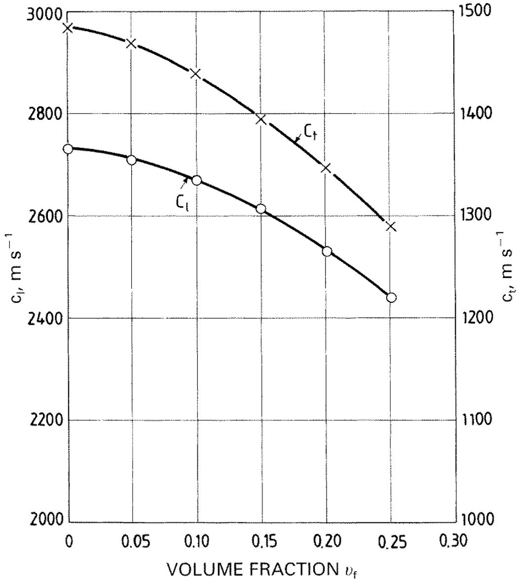
**2 Variation of longitudinal  $c_l$  and transverse  $c_t$  wave velocities versus filler volume fraction  $v_f$**
