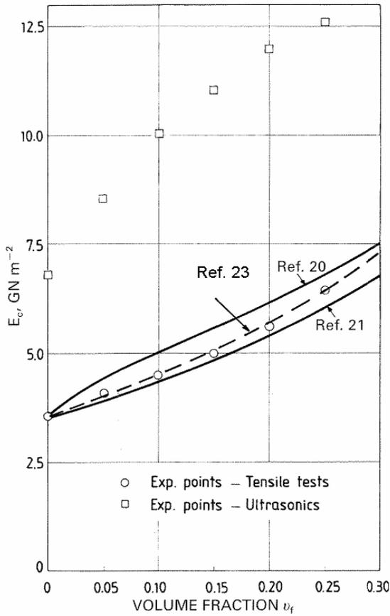
6 Variation of elastic modulus  $E$  versus filler volume fraction  $v_f$  obtained from tensile experiments; comparison with values obtained from ultrasonic experiments
