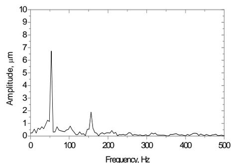
Fig. 4. Spectrum of signals that are obtained measuring rotary system with bearings of sliding, clearance is 50 μm, frequency of rotor revolution 3000 rev/min
