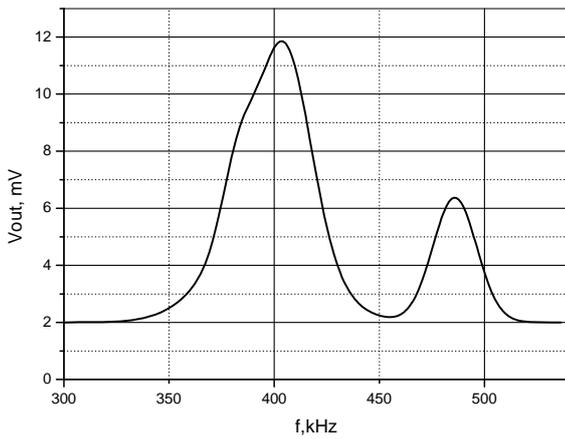
Fig. 6. Air coupled transducers pair transmission AC response
