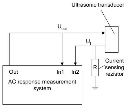
Fig. 7. Transducer impedance AC response measurement setup
