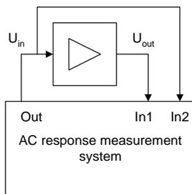
Fig. 2. Ultrasonic preamplifier AC response measurement setup
