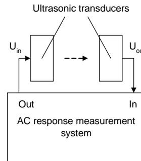
Fig. 5. Transmission AC response measurement setup
