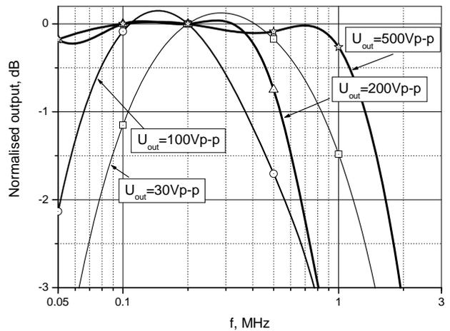
Fig. 9. Frequency response for IRFZ34N configuration
