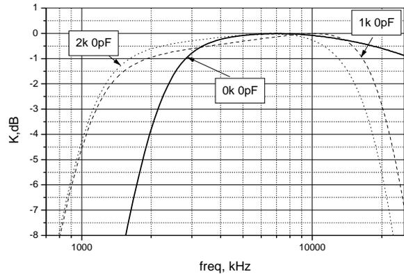
Fig. 4. Low noise preamplifier AC response at various design stages
