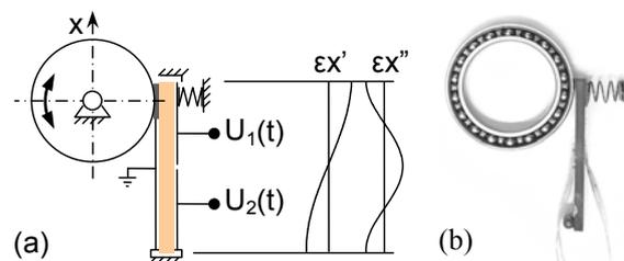
Fig. 1. Inertial piezomotor's schematics (a) and prototype (b)
