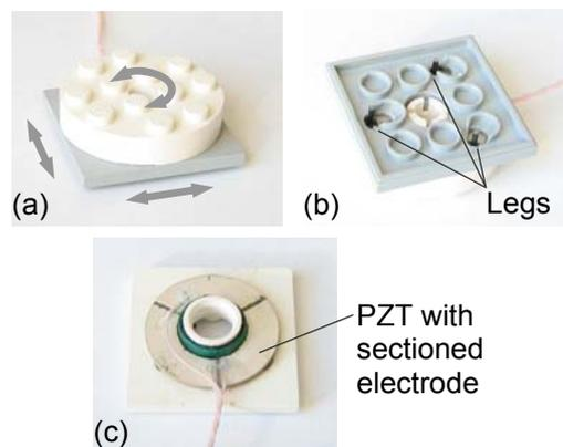
Fig.6. Top (a), bottom (b) and setup (c) views of the three degree-of-freedom "smart" brick
