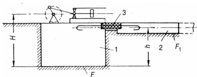
Fig. 1. Diagram of the foundation with the hinge-joined massive plate: 1 – foundation; 2 – plate; 3 – swivel link
