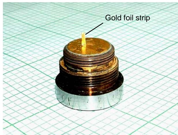
Fig. 11. Thick protector with the diffusion bonded piezoelement and gold foil strip
