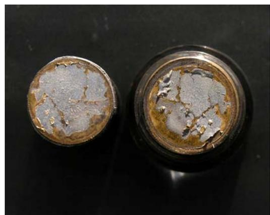
Fig. 13. Delaminations in bismuth titanate piezomaterial when the pressure or/and the temperature were too large for this piezoelectric material. In a tensile strength
