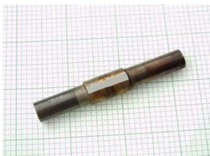
Fig. 7. The bonded stainless steel rods
